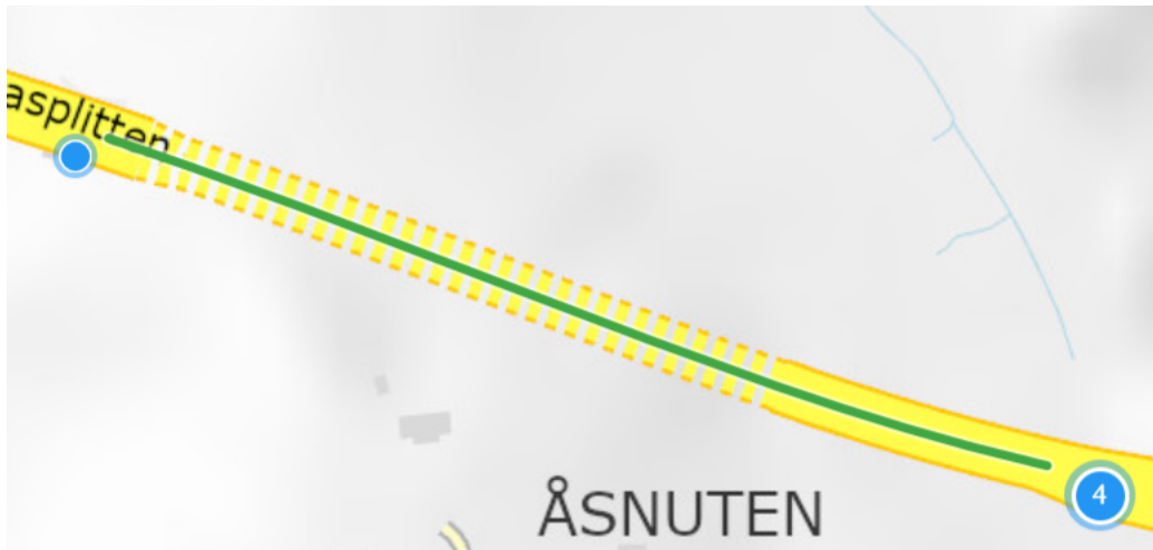
Figure 36: A tunnel tube (green) with two associated "skiltpunkt" (blue) positioned outside the tunnel
