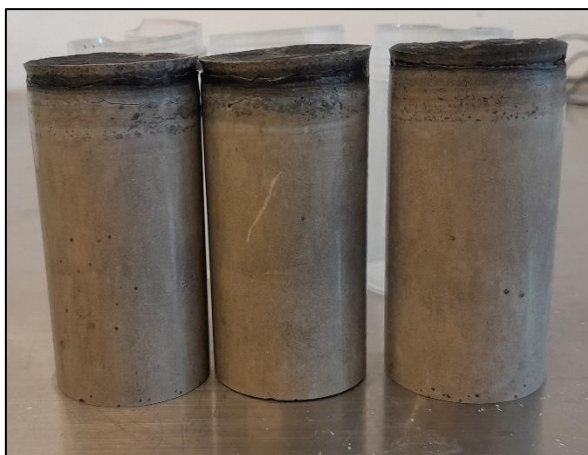
Figure 4. 4 Reference (GP) plugs out of the oven (7 days, 62°C) before polishing
