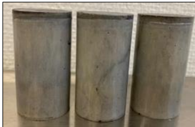
Figure 4. 2 Reference (GP) plugs out of the oven (4 days, 62°C) after polishing
