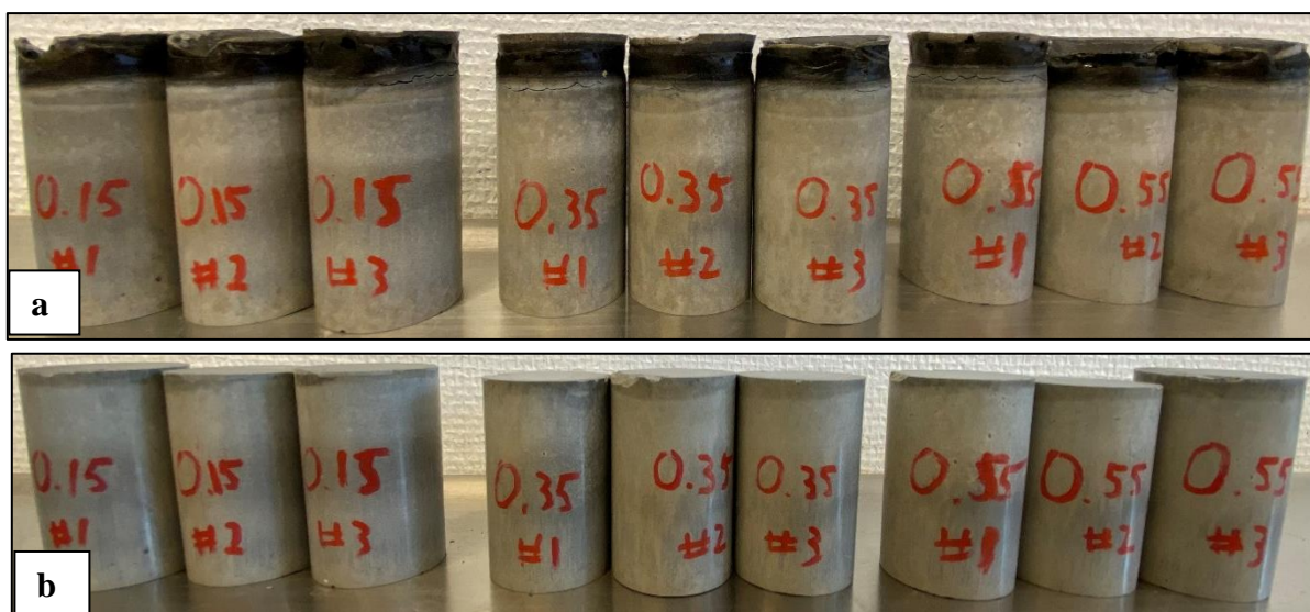
Figure 4. 10 Plugs out of the oven (4 days, 62°C). a) Before polishing. b) After polishing
