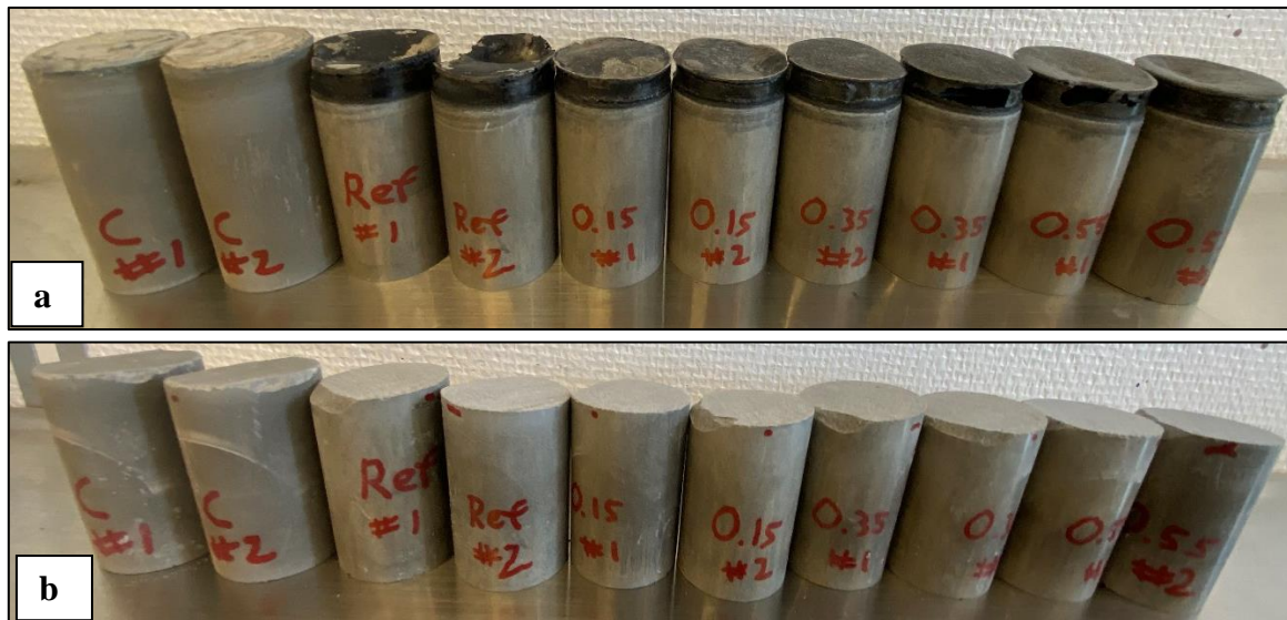
Figure 4. 12 Plugs for fluid absorption, a) before polishing, b) after polishing
