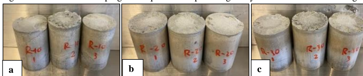
Figure 4. 7 Plugs out of the oven (4 days, 62°C) after polishing. a) 10g Quartz. b) 20g Quartz. c) 30g Quartz
