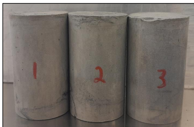
Figure 4. 3 Reference (GP) plugs out of the oven (10 days, 62°C) after polishing
