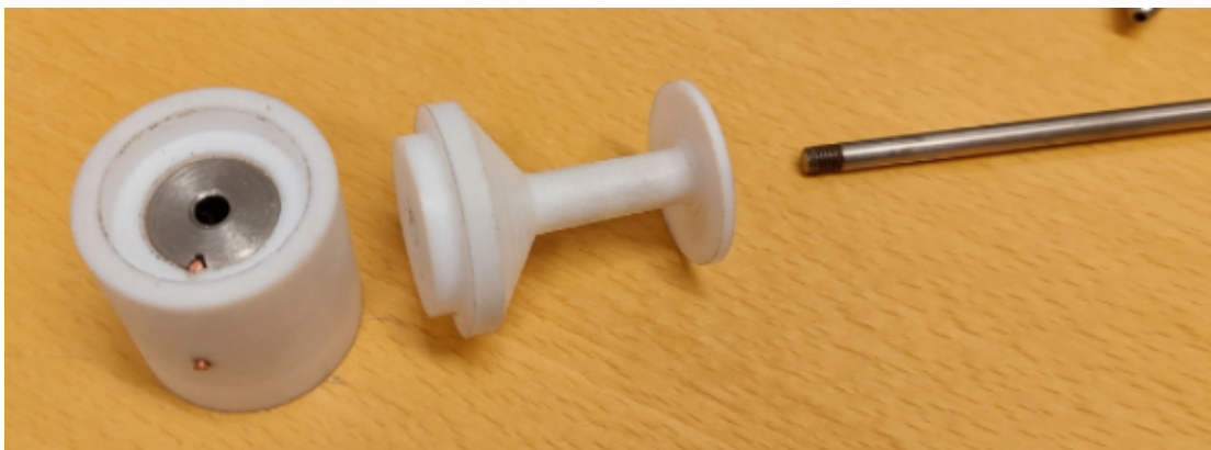
Figure 3.17 - Picture of the final product of the PTFE isolated modified bob
