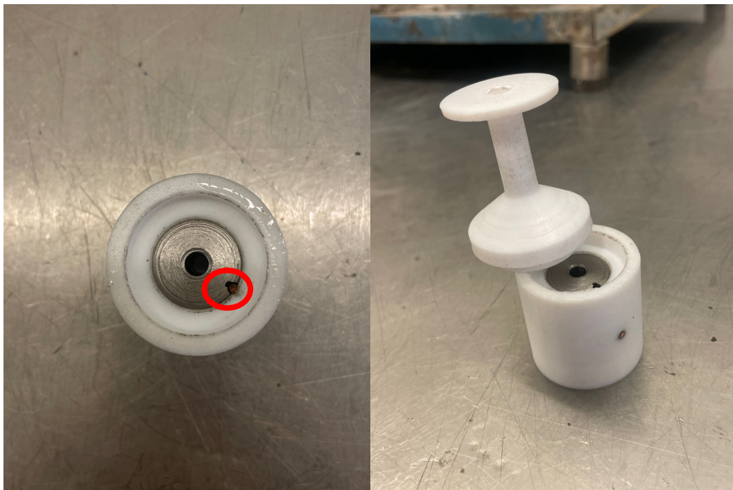
Figure 3.8 - Modified bob, where the inner copper wire is circled
