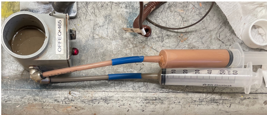
Figure 3.12 - Modified Thermo-cup with the syringes connected to it through tubes
