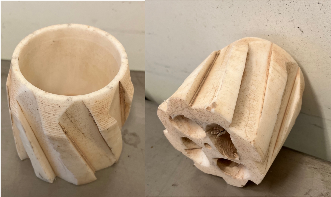
Figure 3.9 – PTFE modified propeller
