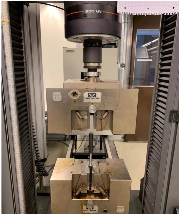
Figure 27: Lowering the upper part of the machine to specimen.
