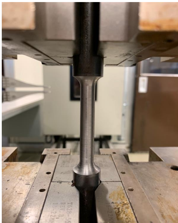
Figure 28: 1 cm protruding on both ends and tightened grips.
