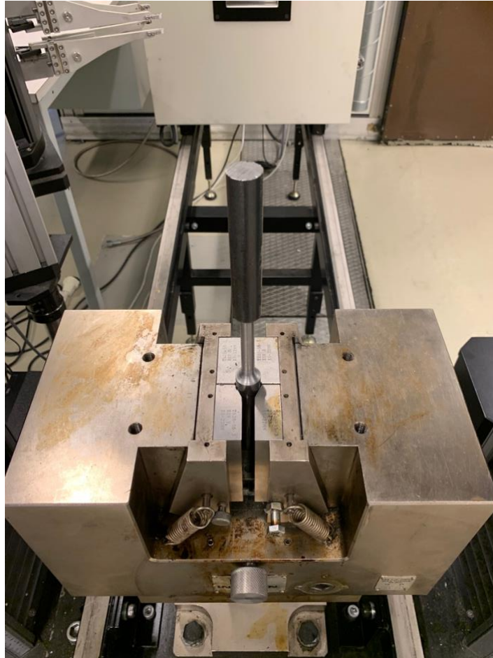
Figure 26: Installing the specimen to bottom grips.
