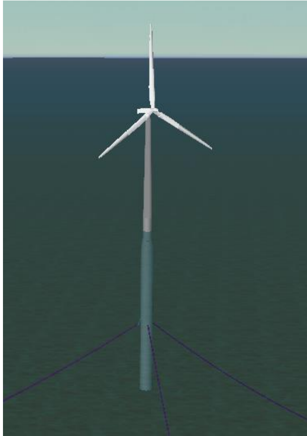
Figure 3-1: OC3-Hywind FOWT OrcaFlex model.
