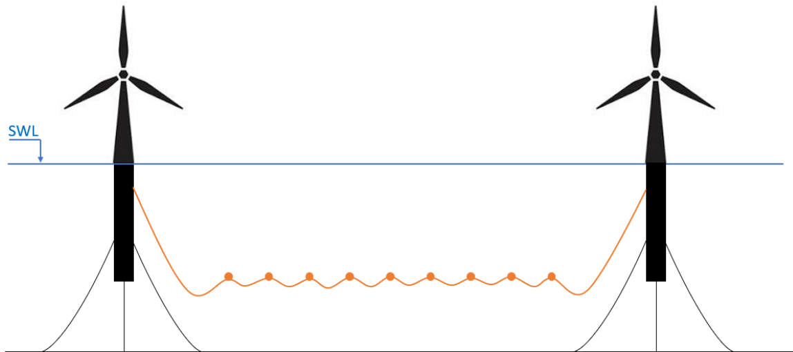
Figure 5-7: Concept of two FOWTs with a suspended power cable.
