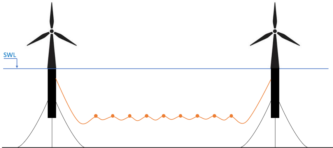
Figure 3-6: Concept of two FOWTs with a suspended power cable.
