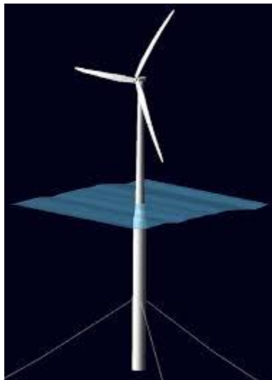
Figure 2-5: OC3-Hywind 5 MW FOWT (reproduced from Jonkman (2010)).
