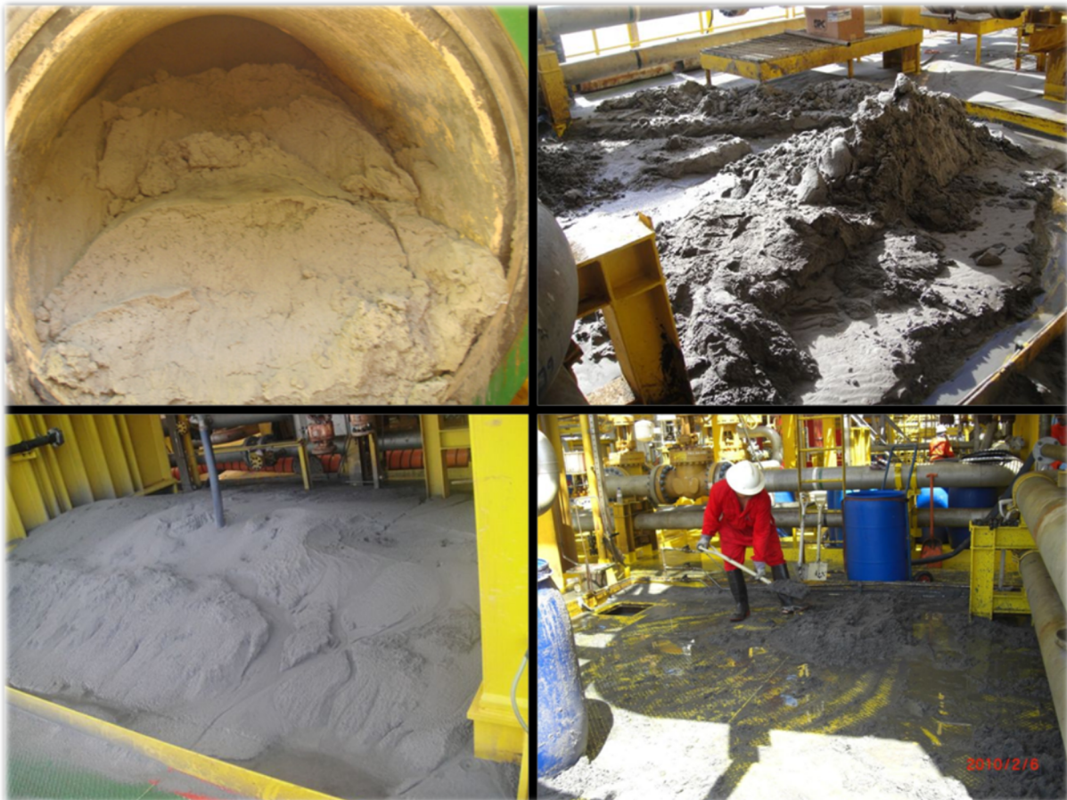
Figure 6: Issues caused by sand production (eProcess Technologies)
