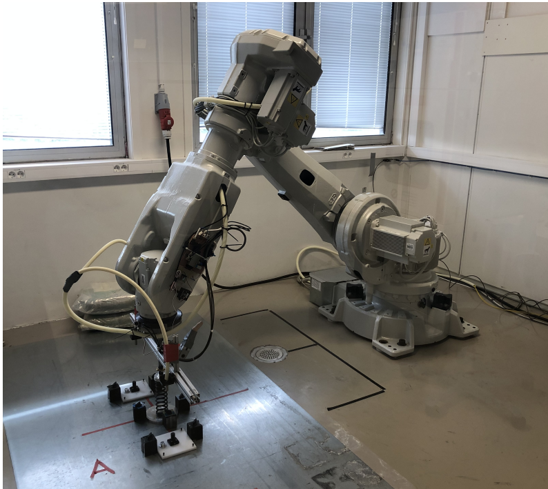
Figure 1.2: ABB IRB 6620 Industrial Robot Manipulator used at Laerdal Medical. The robot is in the testing configuration using a spring in place of a test object.
