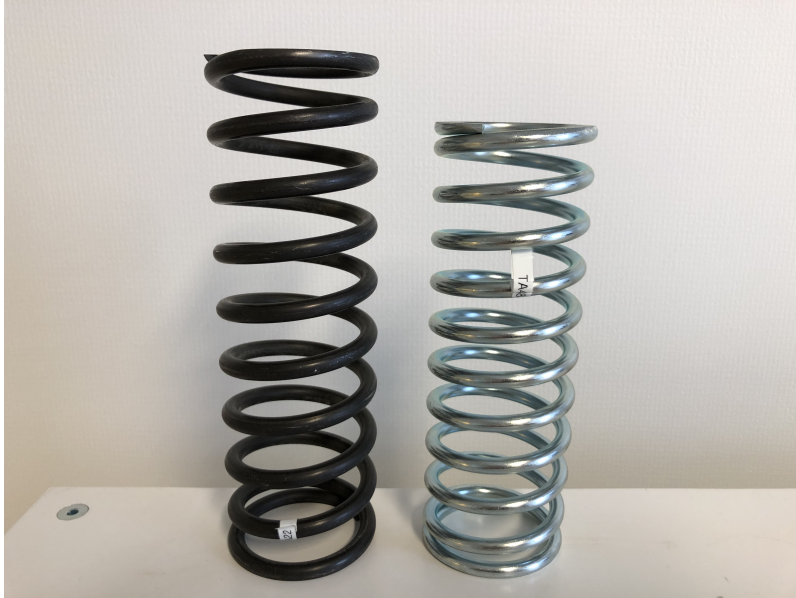
Figure 3.9: Springs used for compression testing.
