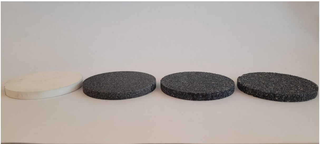
Figure 4-OFITE ceramic discs. From left to right: 10 \mu\text{m} , 50 \mu\text{m} , 120 \mu\text{m} and 160 \mu\text{m} .
