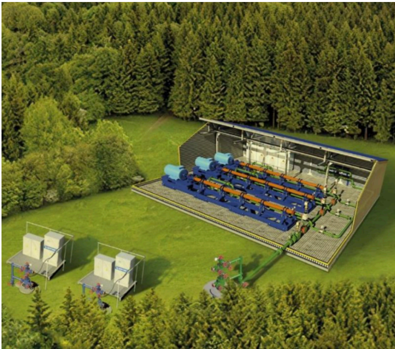
Figure 3.3 – Block pumping station
