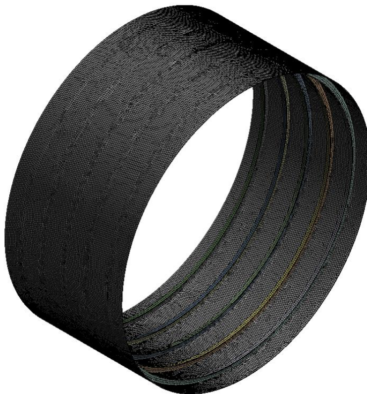
Figure 6.8: 3D ANSYS model showing fine mesh
