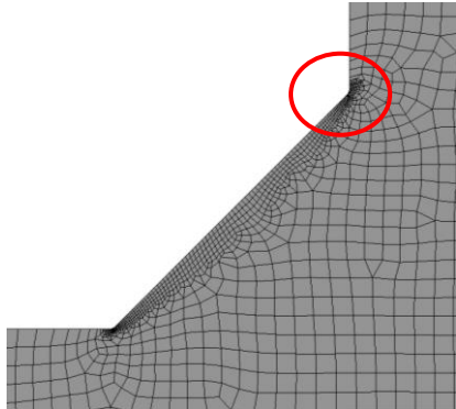
Figure 6.5: Mesh convergence study for 2D axisymmetry model - Mesh refinement model and corresponding max. equivalent stress at welds
