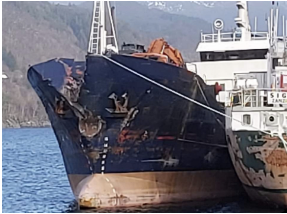
(a) Vessel Tornado after collision
