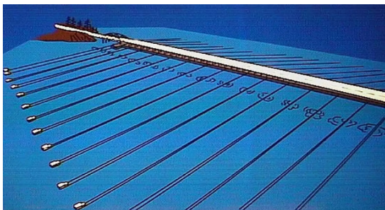
(a) Longitudinal continuous pontoons. Adapted from [19].
