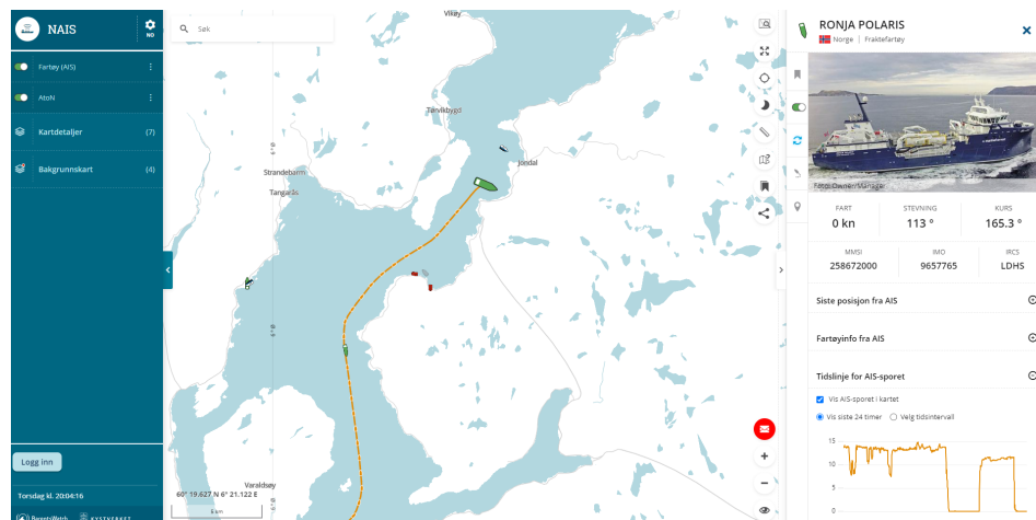
Figure 2.5: AIS data example from Kystverket.no showing real-time positioning of the wellboat Ronja Polaris.
