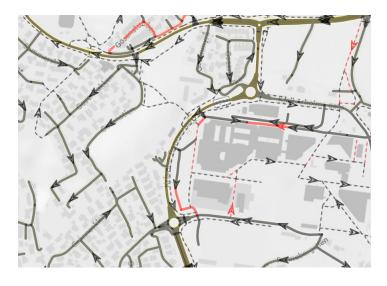
Figure 35: Some "veglenker" highlighted in Vegkart, along with arrows indicating their direction
