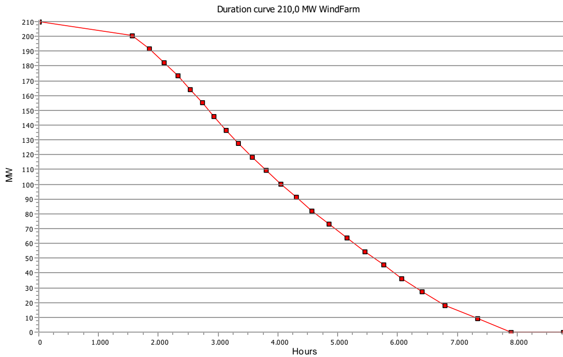
Figure 48: PARK time varying AEP using scaled ERA5, corrected power curve and Eddy viscosity wake model. Figure displays the duration curve of the 210 MW wind farm consisting of 35 turbines. The results includes wake losses and any curtailment losses.
