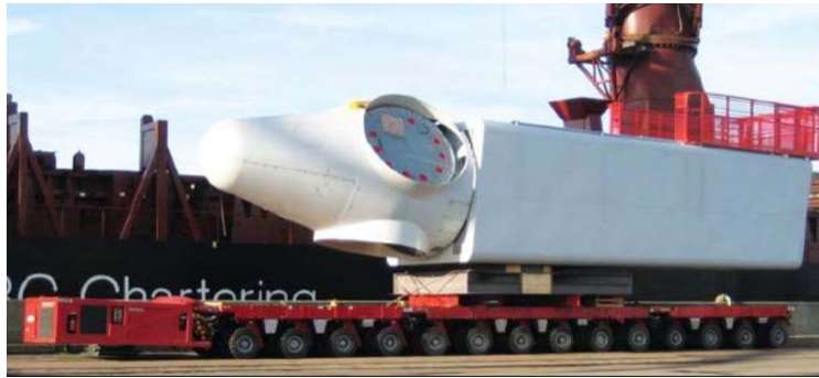
Figure 24. SPMT carrying the nacelle and the hub [28].
