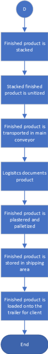
Figure 9 Packaging manufacturing process flowchart B
