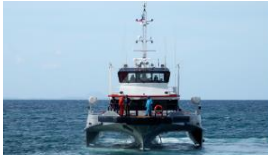
Figure 4.2: Trimaran SWATH vessel. [97]
