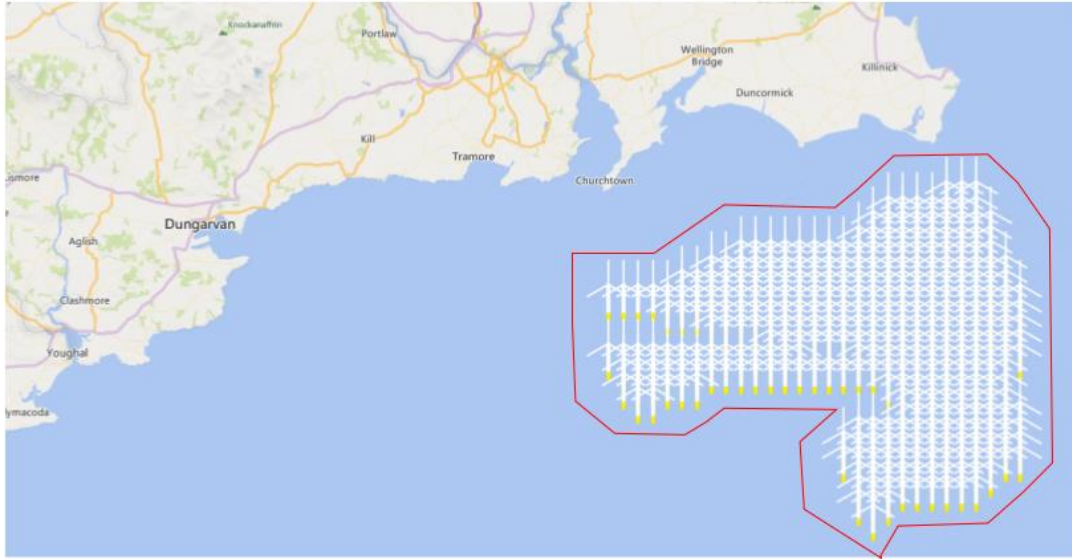
Figure D.5: Ireland`s Array, total capacity: 5.2 GW.
