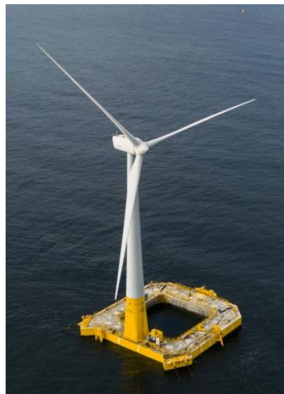
Figure 2.24: Barge-type offshore wind turbine floater. [39]
