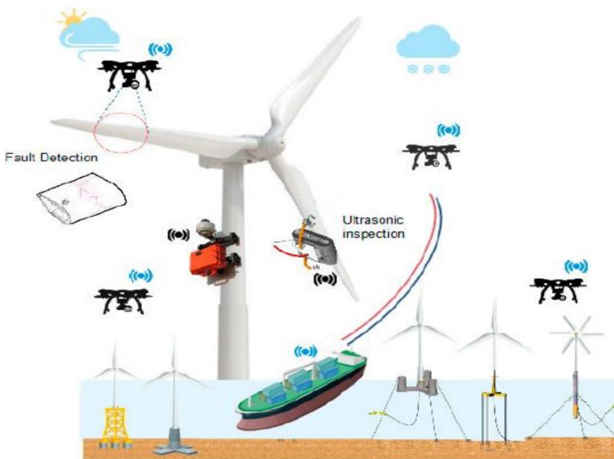
FIGURE 17. INSPECTION OF WIND FARM BY ROBOTICS [51].
