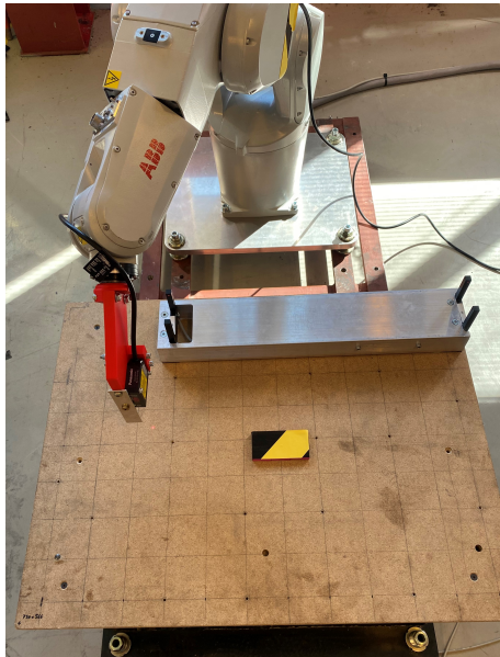
Figure 9: Work environment with the robot, the tool with sensor, and the box step in the middle of the table.
