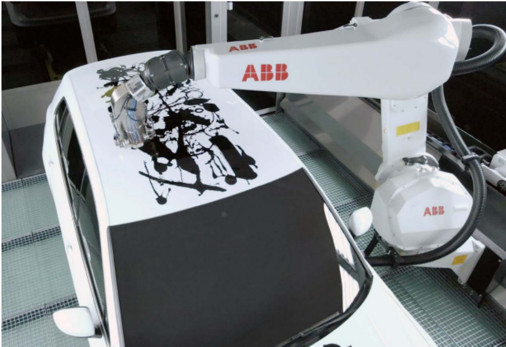
Figure 1.1: Picture of custom car paint using PixelPaint. Figure provided by ABB robotics Pixel Paint manual, page 1 [3].
