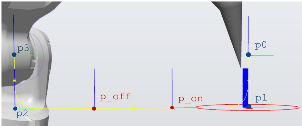
Figure 4.1: Robot path for position test, shown in RobotStudio simulation tool.
