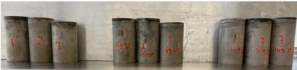
The diagram shows plugs containing SP which have been properly polished and ready for testing
