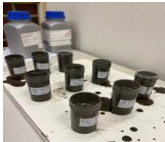
Figure 3.18: Geopolymer slurry filling in plastic mould
