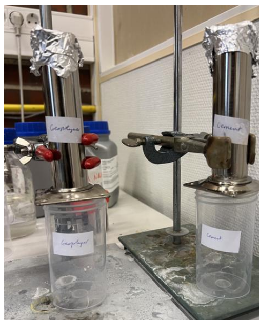
Figure 3.15: Leakage test setup
