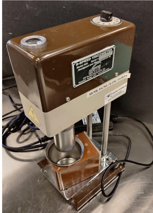
Figure 3.12: OFITE viscometer used to measure the rheology of geopolymer cement slurry.
