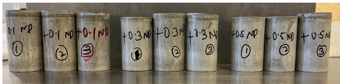
The diagram shows plugs containing NP which have been properly polished and ready for testing
