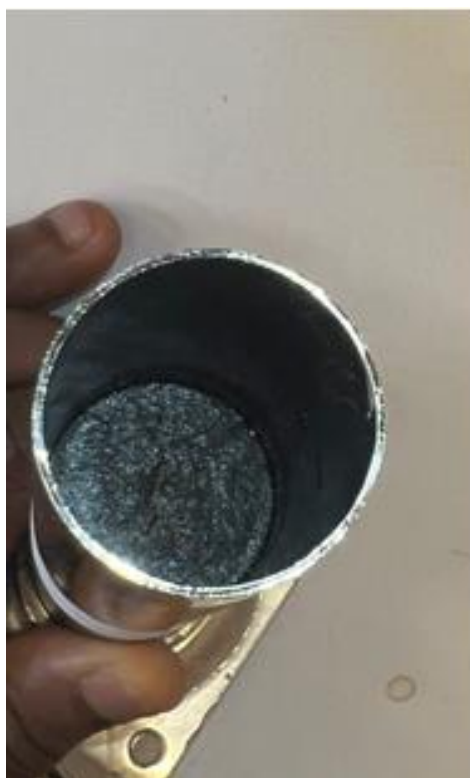
The diagram shows the condition of the cement plug after the complete leakage test cycle
