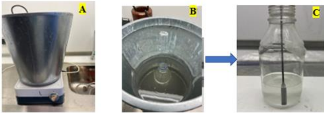
Figure 3.17: A) Heat bath setup. B) Liquid sodium metasilicate deeply immersed in the hot water bath C) Crystal clear 40% solution after the heating process
