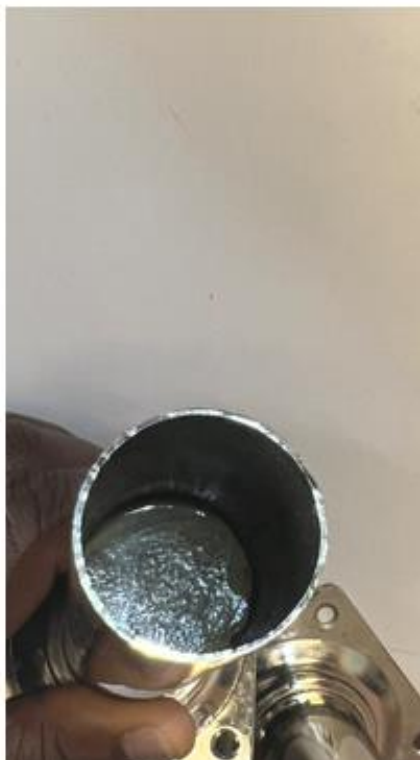
The diagram shows the condition of the cement plug after the complete leakage test cycle
