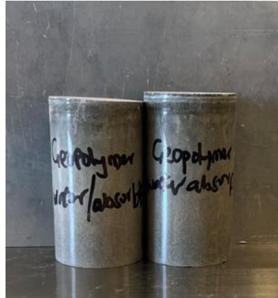
The diagram shows polished neat geopolymer to be used to test for water absorption
