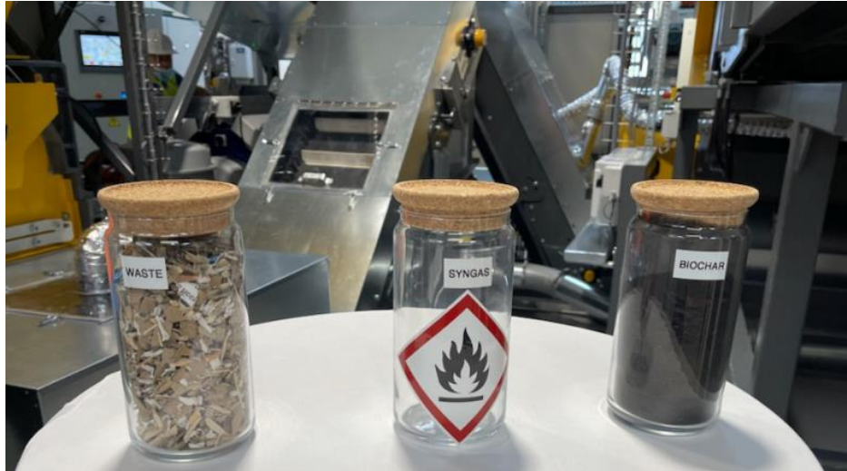
Figure 2: picture showing waste feedstock and pyrolysis products biochar and bio-gas (syngas) (Vow ASA, 2021)
