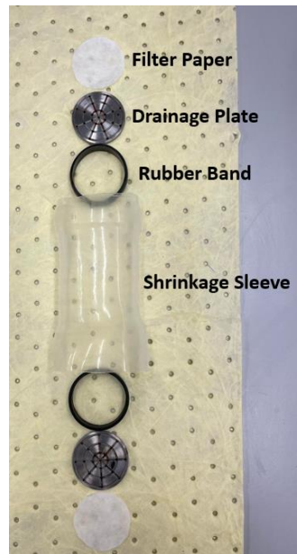
Figure 3.10 - Core preparation setup
