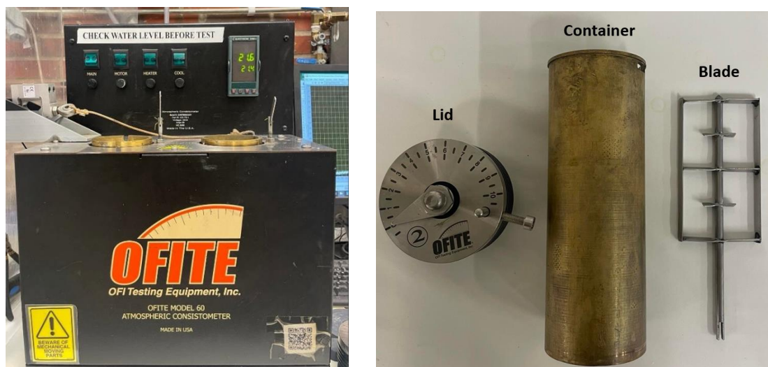
Figure 3.3 - Consistometer (left) and container setup (right)
