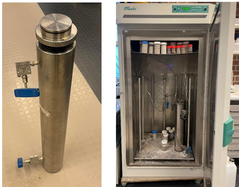
Figure 3.5 - Autoclave (left) and curing oven (right)
