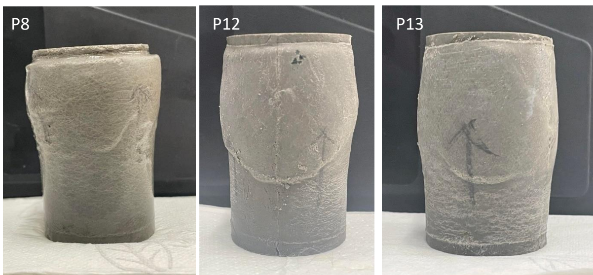
Figure 4.31 - State of core samples after testing
