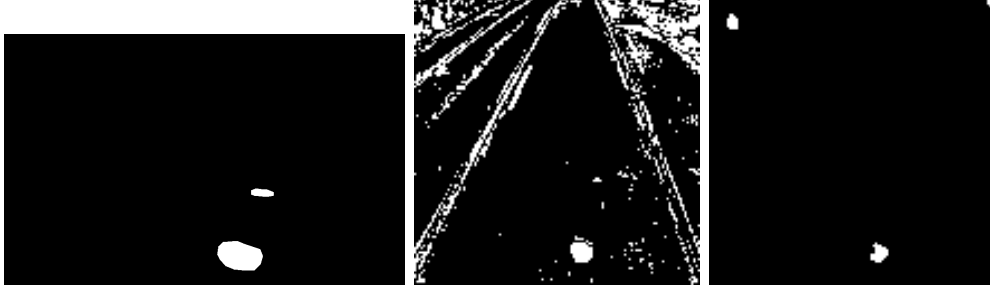
Figure 6.1: Mask image of pothole vs localization of pothole using VAE model
