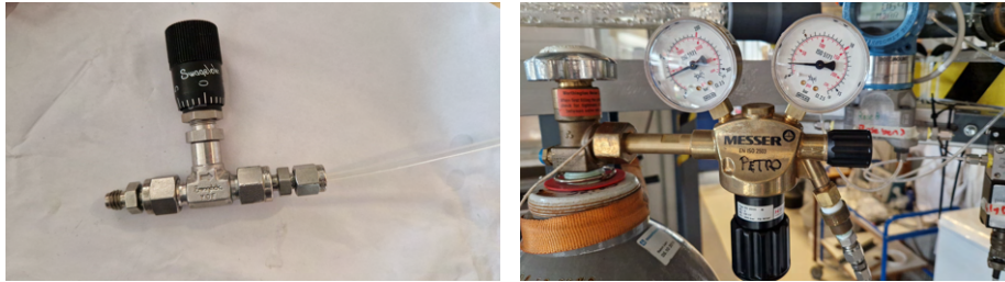
Figure D.3: valve and regulator used to control flow
