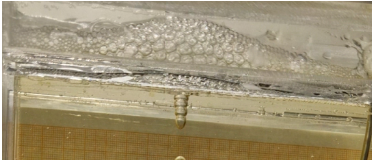
Figure 4.9: Foam accumulation at the surface of 1.00% HEC fluid
