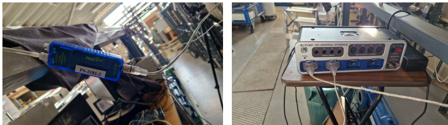
Figure D.5: Pasco pressure sensor and universal interface
