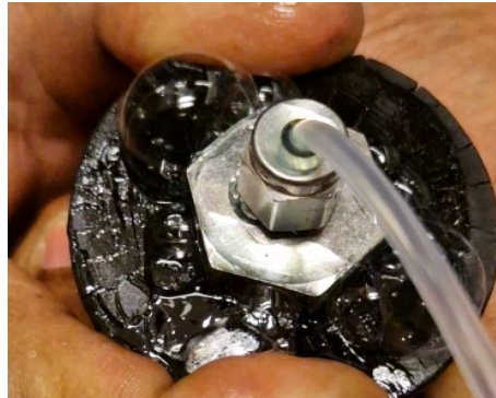
Figure C.2: Leak from cork at preliminary testing
