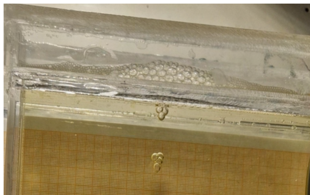
Figure 4.6: Foam accumulation at the surface of 0.75% HEC fluid
