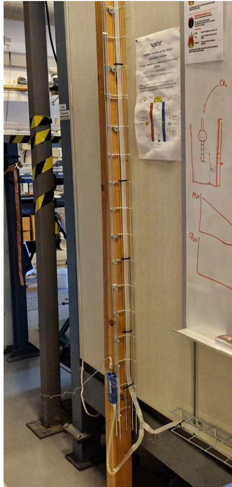
Figure C.4: Calibrating sensor using hydrostatic pressure
