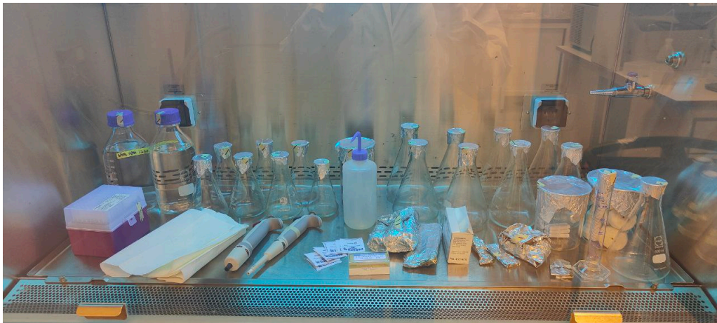
Figure 3.2: Equipment placed in the closed cabinet for UV exposure
