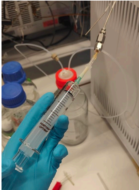
Figure 3.11: Insert the gas through a metal inlet tube immediately after extracting gas to prevent gas contamination
