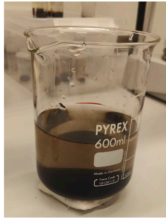
(b) Step 2 - Fe_3O_4 extraction from liquid using a magnet
