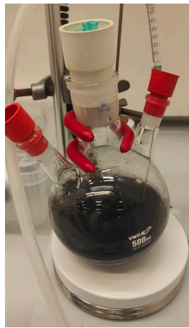
(a) step 1 - Fe_3O_4 solution in 3 neck round bottom flask
