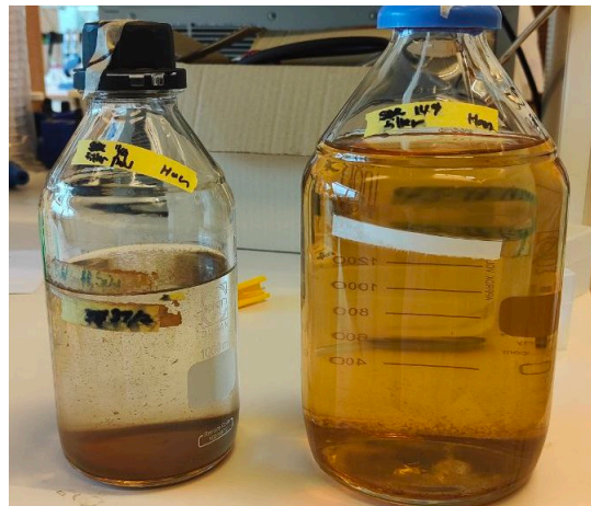
Figure 4.12: PW_{WW} (Left) and SBR_{WW} (Right) after autoclaving. PW_{WW} looked clear while SBR_{WW} showed orange and slightly brown in colour. Particles could be seen suspended in both mediums, with more over in PW_{WW} .
