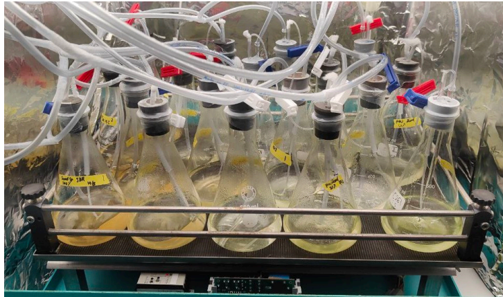
Figure 3.5: WW experiment setup in the incubator in the incubation cabinet with additional air pump and controlled condition.
