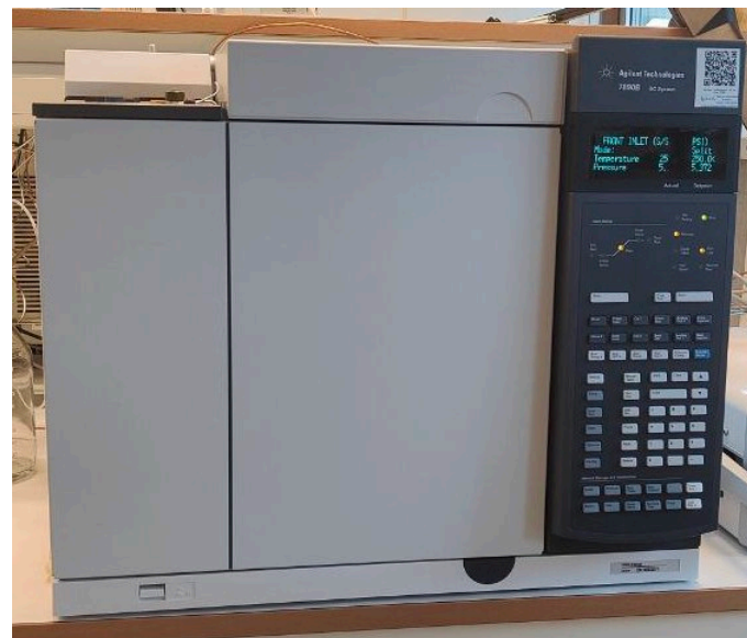
Figure 3.10: Gas chromatography on BMP bottles was analysed using Agilent Technologies 7890B GC system
