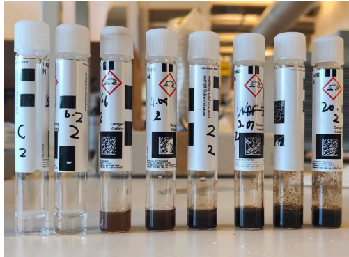
Figure 3.7: NP after sonication lined up in increasing concentration from left to right
