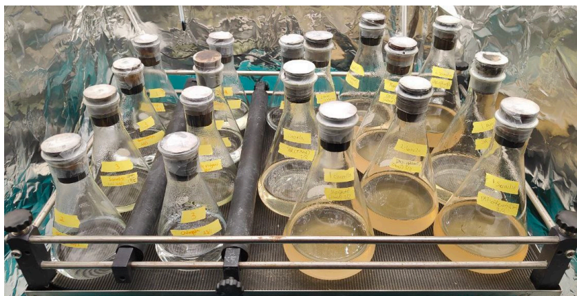
Figure 3.4: Scenedesmus sp. cultured with WW as growth media in an incubation cabinet with a controlled condition. This was to allow microalgae to adapt to individual WW
