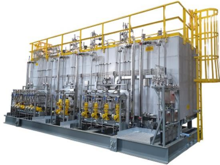
Figure 17: Chemical injection package [58]
