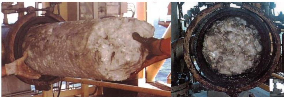
Figure 14: Formation of hydrates in pipelines [48]
