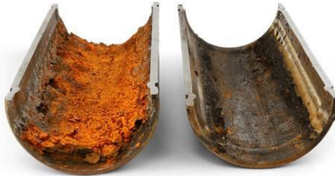
Figure 11: Corrosion formation in pipelines [54]
