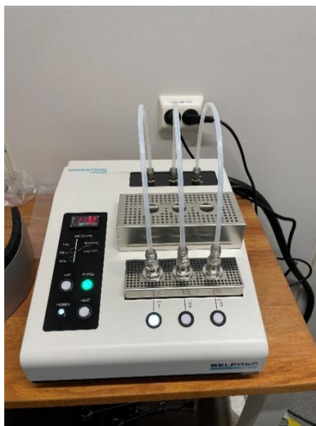
Figure 31. BELPREP external degassing unit (at UIS)
