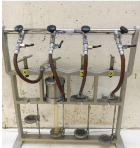
Figure 3.11: API filter press
