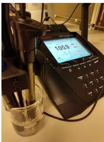
FIGURE 2, NO 3 -ISE MEASUREMENT DEVICE
