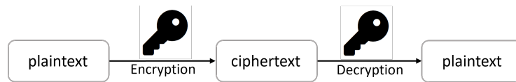
Figure 2.1: A simple sketch demonstrating symmetric encryption and decryption, redrawn from Kessler, G. C. [16]. The same key is used to encrypt the plaintext and decrypt the ciphertext.
