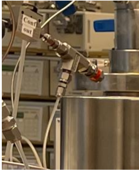
Figure 42 Pressure control valve used to regulate the pressure during heating of confining oil
