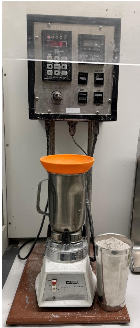
Figure 15 Mixing cup and OFITE Model 20 Constant Speed Blender for cement mixing
