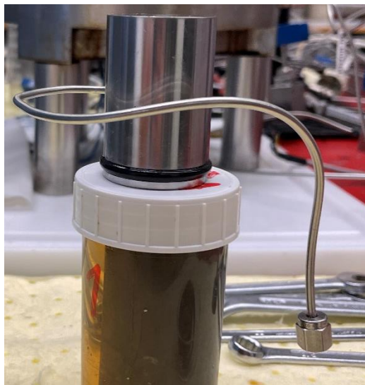
Figure 30 Top of water injection unit
