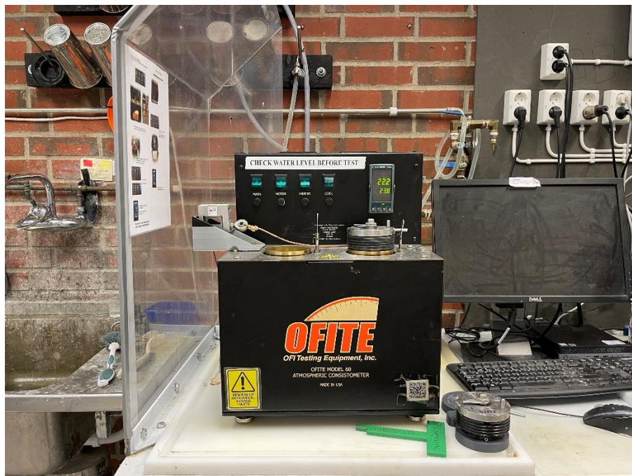
Figure 17 OFITE model 60 Atmospheric consistometer used to condition the geopolymer
