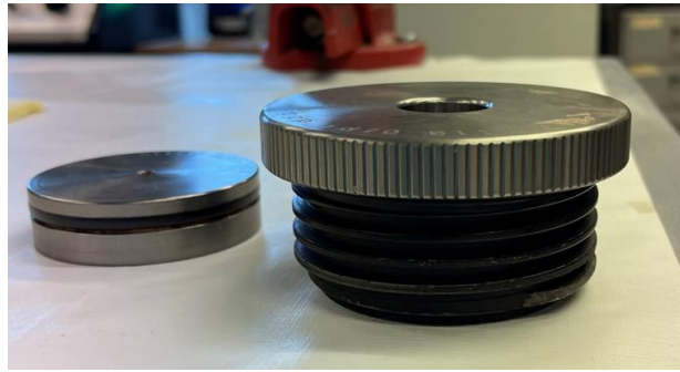
Figure 20 Autoclave cell Inner (left) and Outer lid (right)
