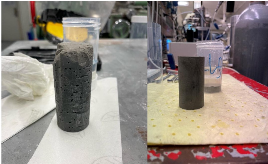
Figure 76 Picture of sample SLL4 (left) after removal from mould and sample SLL8 (right) sample cut and polished
