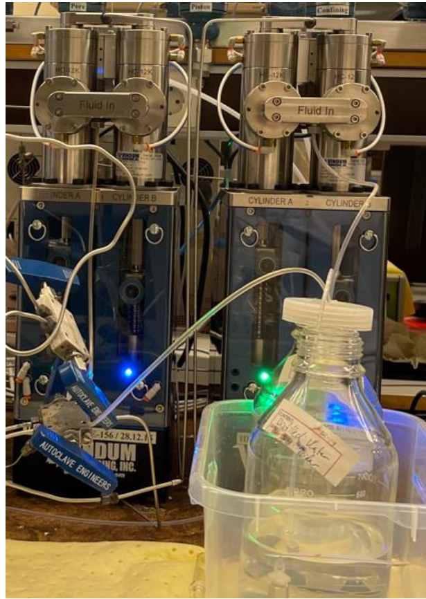
Figure 39 Vidum VP-series High-Pressure Metering Pumps
