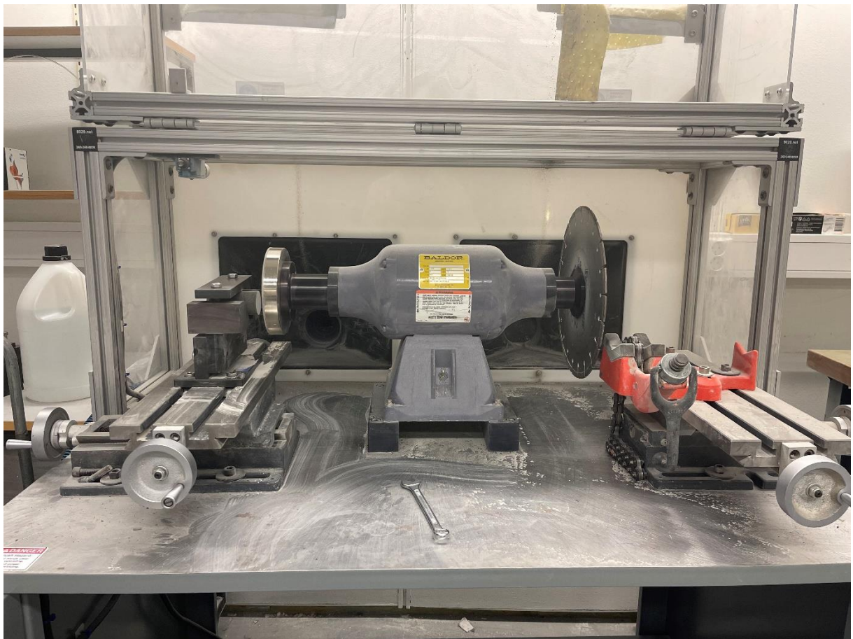
Figure 23 Baldor GCTS RSG-75 cutting and polishing machine
