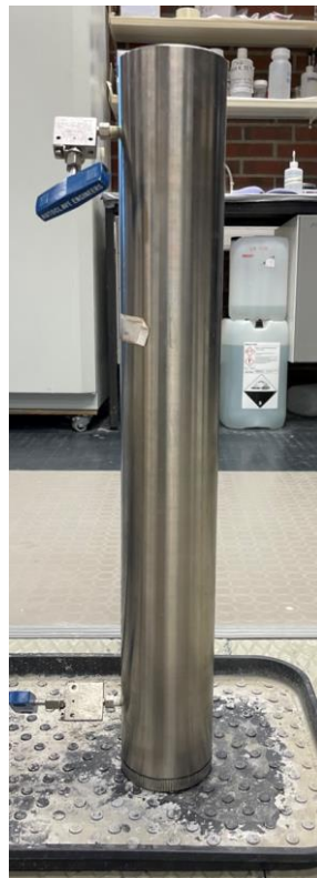
Figure 19 Autoclave curing cell
