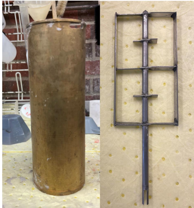
Figure 16 Conditioner cup and mixing blade
