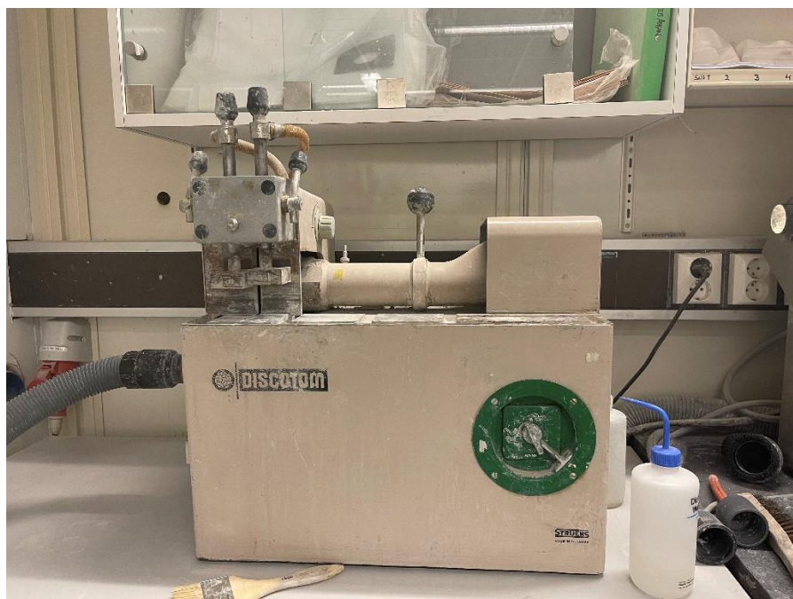
Figure 22 Discotom Cutting machine
