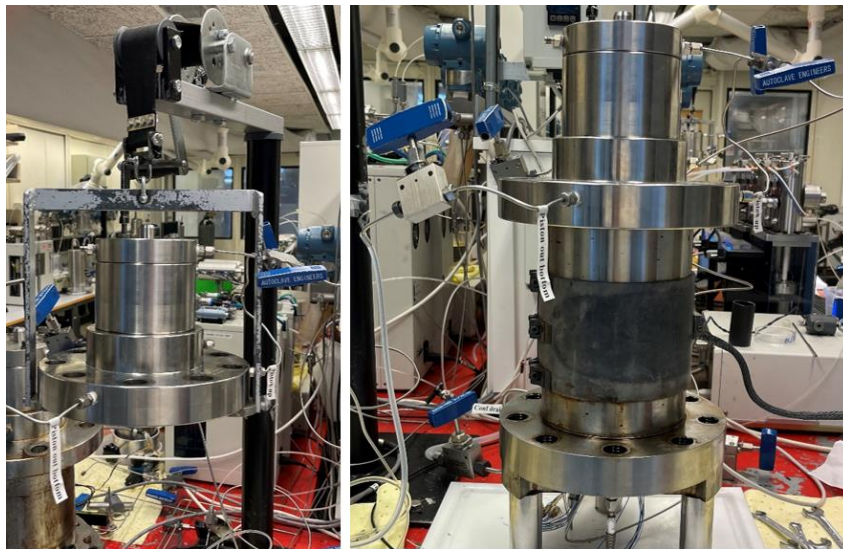
Figure 35 Top of triaxial cell (left) and installed top of the triaxial cell on the confining chamber
