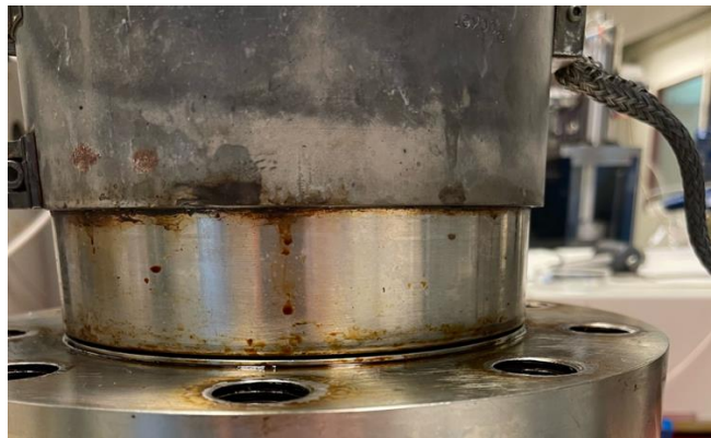
Figure 33 Confining chamber correctly placed on the bottom of the Triaxial cell
