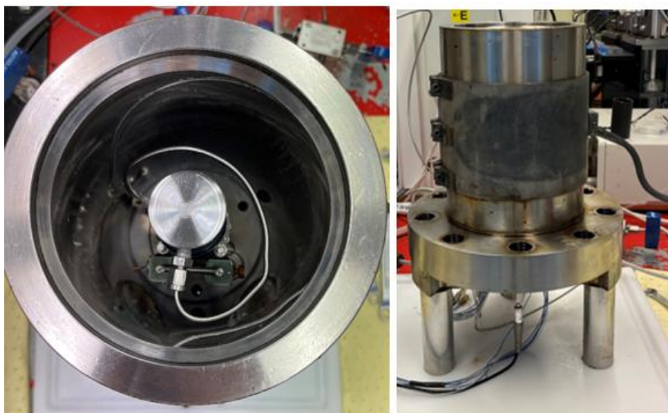
Figure 34 Confining pressure installed, from above and from the side
