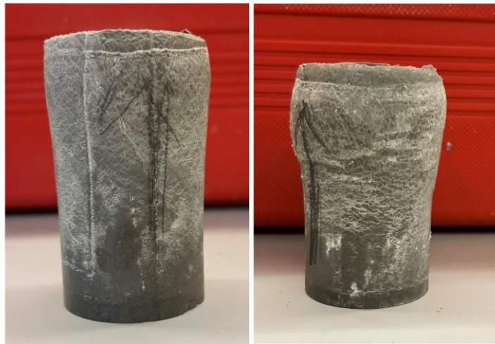
Figure 45 Geopolymer samples after the deviatoric phase (failed samples)
