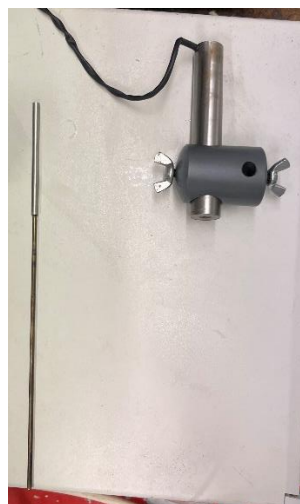
Figure 36 LVDT Axial movement logging equipment
