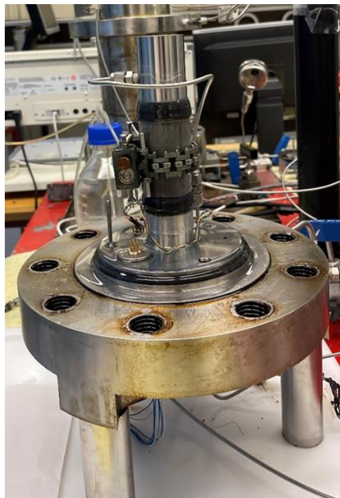
Figure 32 Fully assembled test set-up on the inner part of the confining chamber of a triaxial cell
