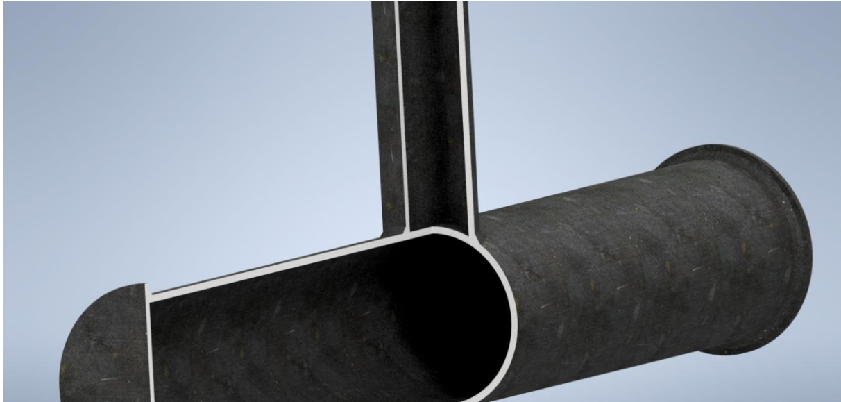
Figure 30 3D model obtained in Autodesk Inventor showing cross-section of weldment to illustrate different tangency angles depending on location.
