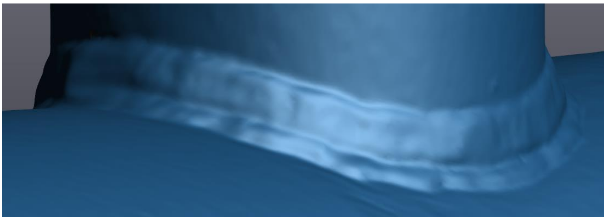
Figure 18 Special attention was paid on scanning the weld surrounding. Mesh is not interrupted in this area.
