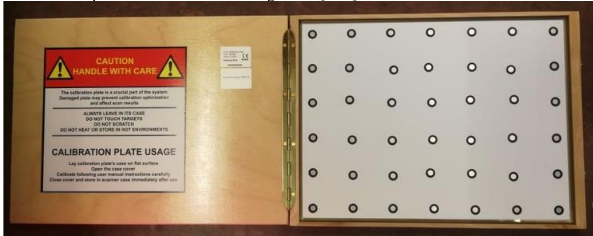
Figure 9 The calibration board - this equipment is delivered with the set of laser
