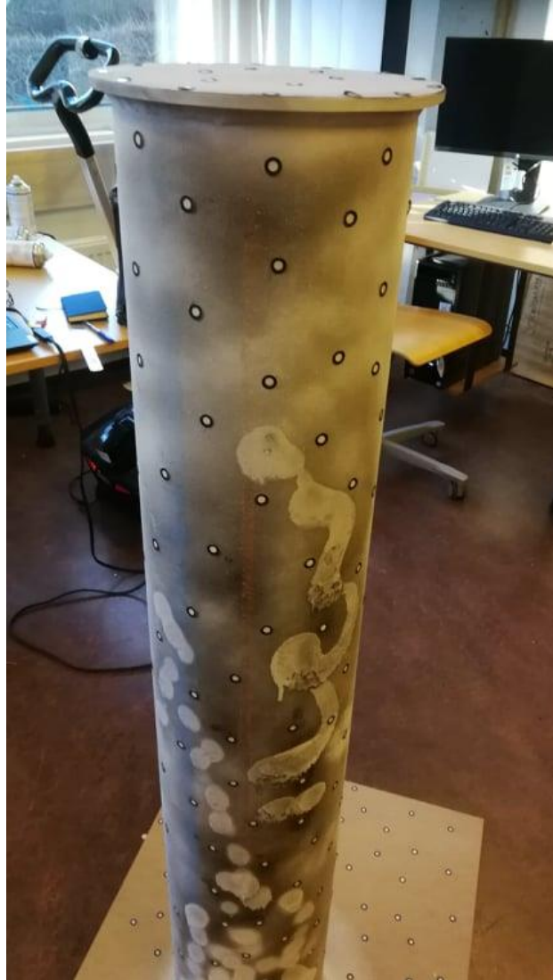
Figure 16 Specimen #2 with concentrated targets count on surface. Average distance 6cm.
