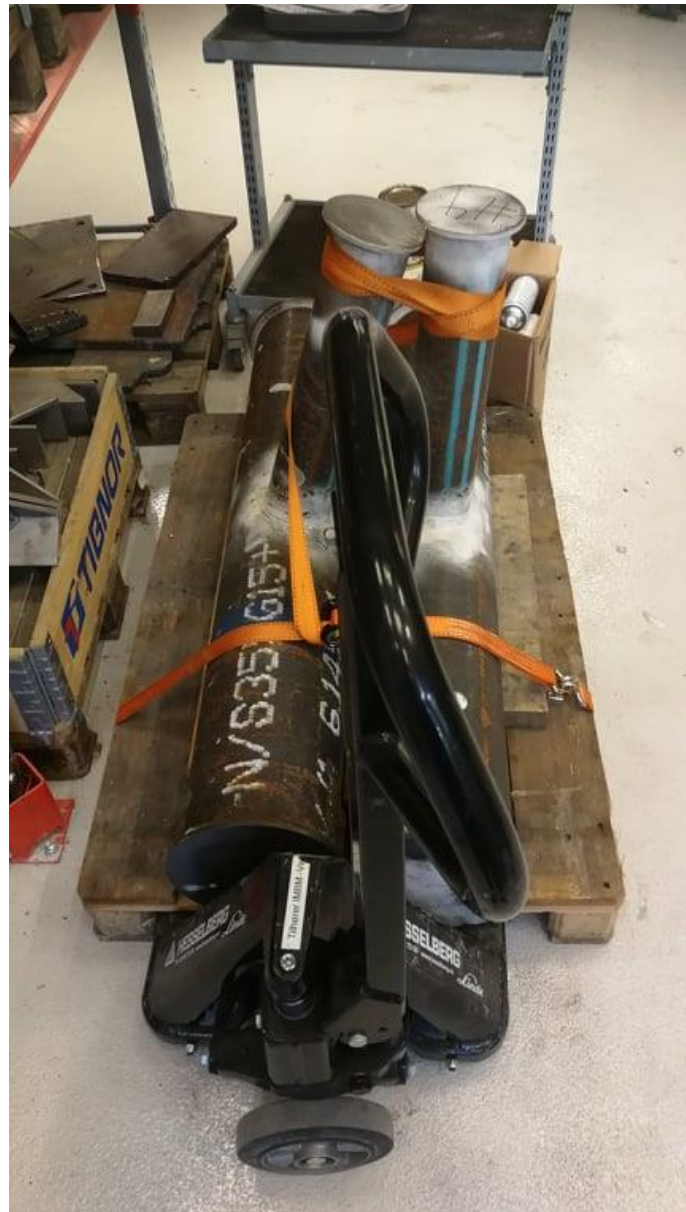
Figure 1 Method of securing the load - specimens - during transportation on cart. Cargo strap and ratchet are used to tie the tubulars tight and prevent them from falling out.
