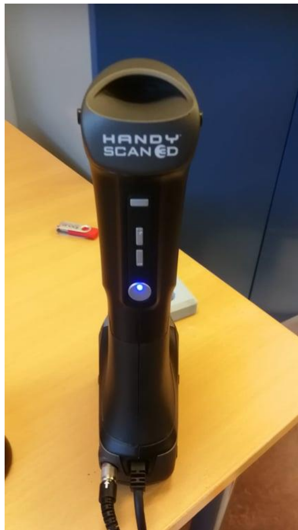
Figure 7 The scanner head connected to CPU and external power source.
