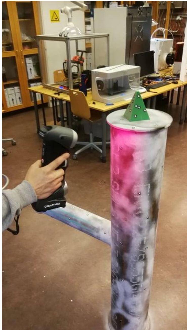
Figure 11 A first attempt to scanning the specimen. Green pyramid on the top helps to initiate scanning with its dense targets pattern. It was also used for size references and quick scanner/application checks.
