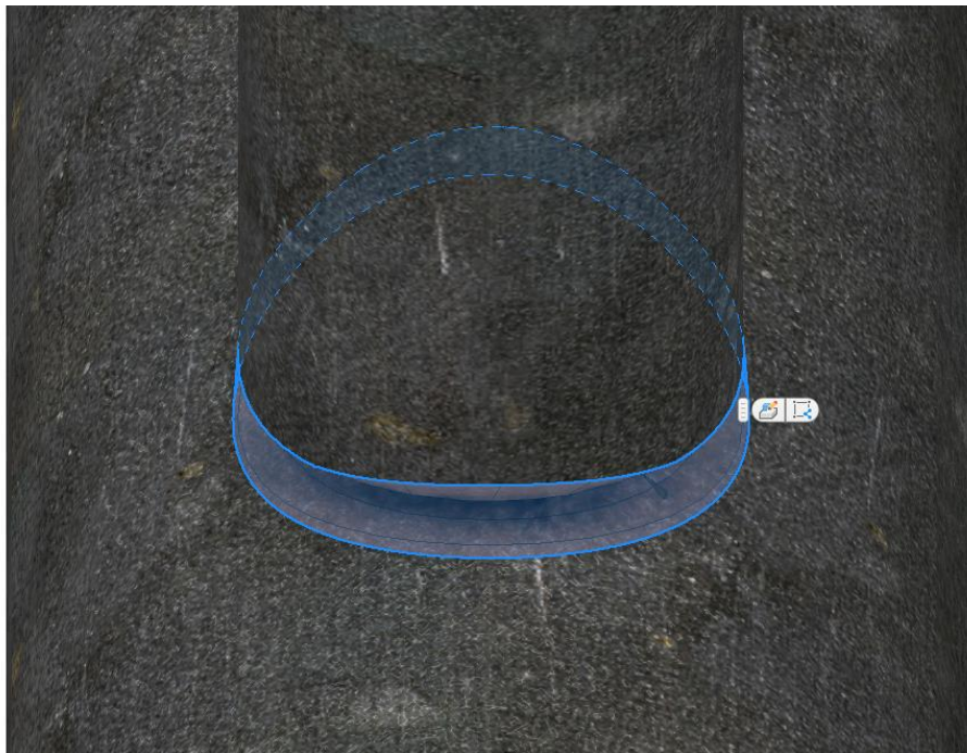
Figure 44 The weld surface eventually obtained in 3D model. The surface was then 'Stitched up' with surrounding surfaces and 'sculpted' into Inventor solid model.
