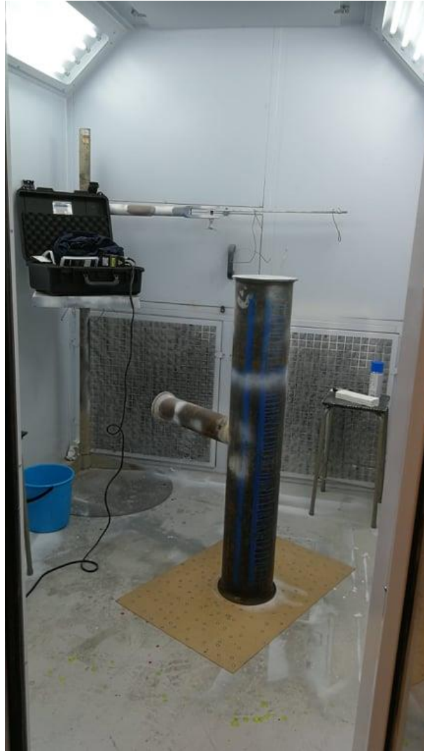
Figure 17 Specimen #5 in the university paint booth before preparation (paint and targets). The main mechanical ventilation inlet filters visible in the background.
