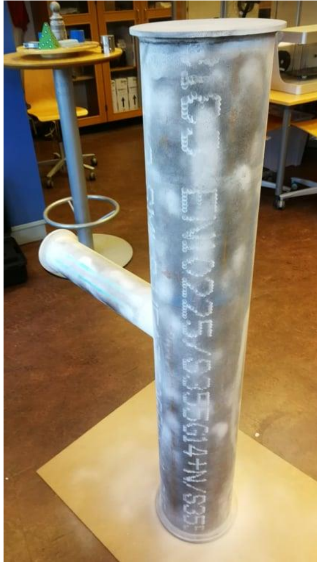
Figure 15 Specimen #1 painted white. The manufacturer markings are still visible under the AESUB coat.
