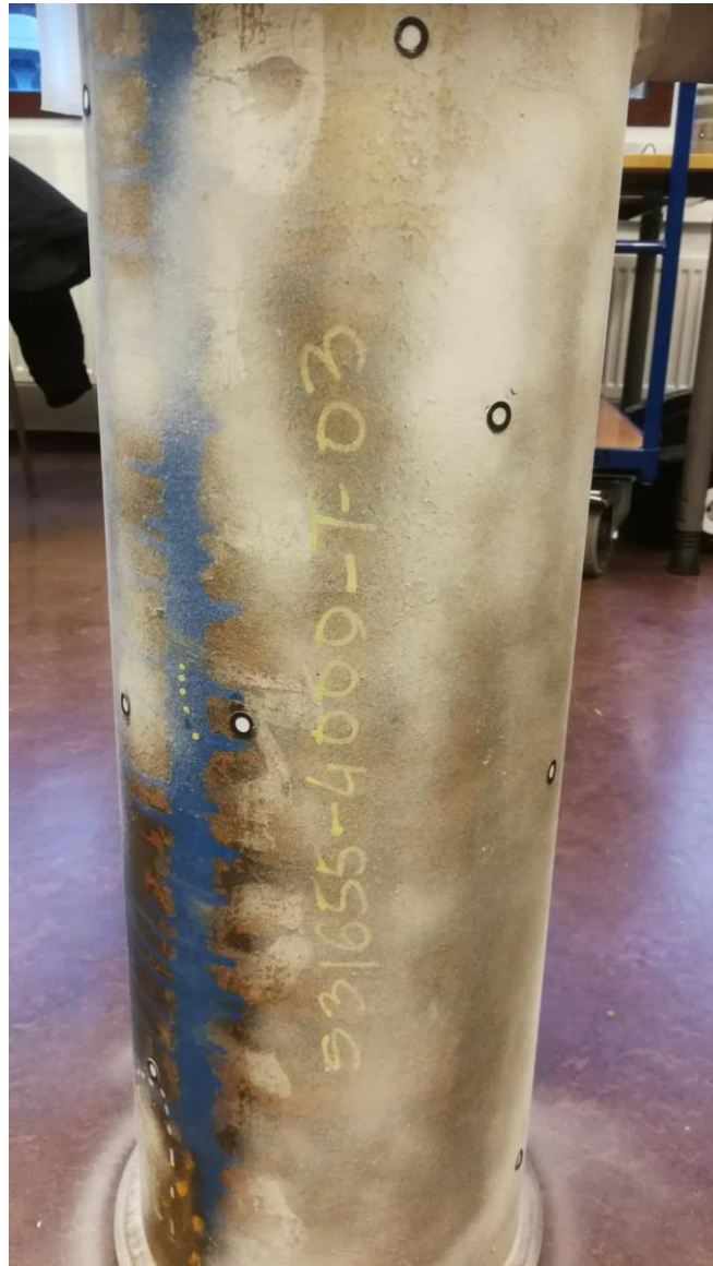
Figure 13 Not painted specimen. Visible the targets for reference patterns, stains, manufacturer markings and numbers of different colours - making difficulties on surface gathering.
