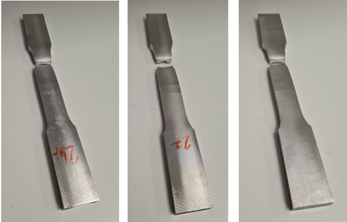
Figure 30 The tension specimens after the tests were done.
