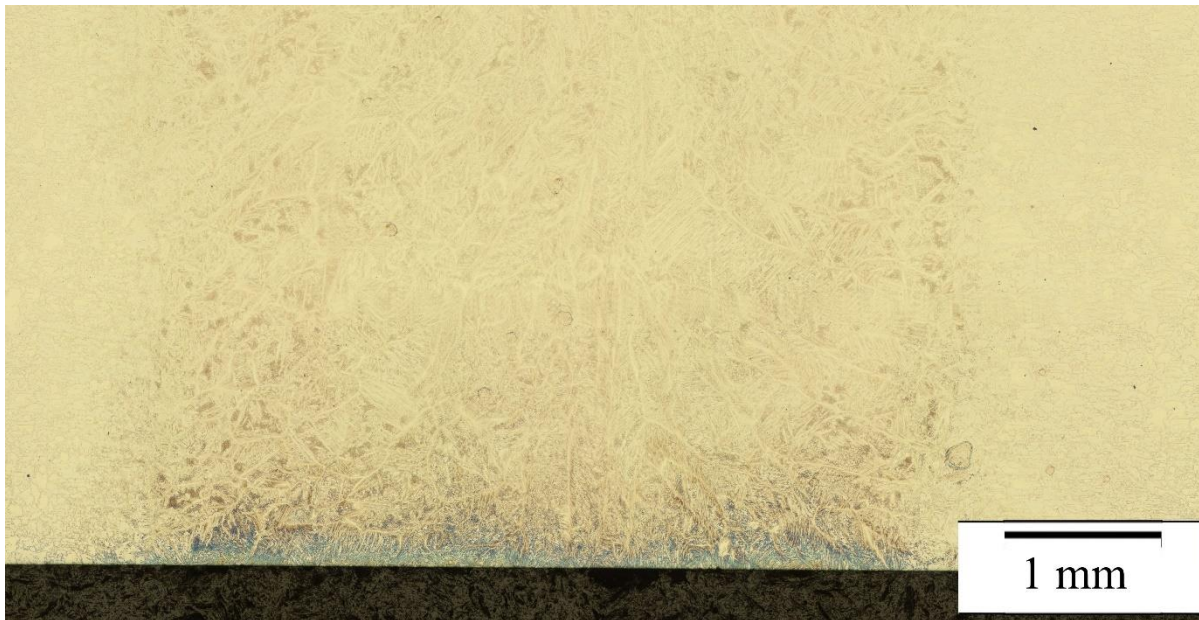
Figure 17 Zoomed in version Figure 16 showing the edge of the sample. It shows some allotriomorphic austenite.
