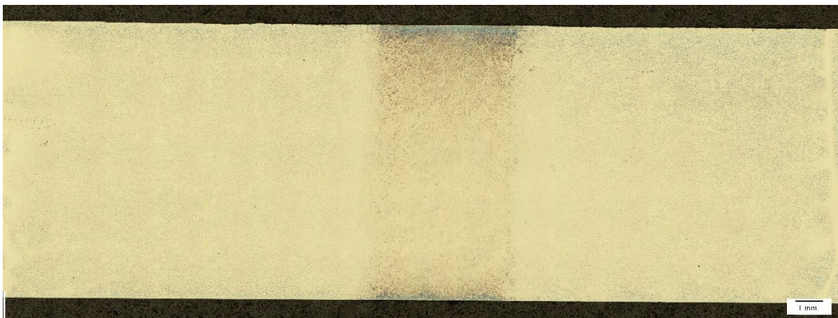
Figure 16 Overview of the Bottom-view sample. The edges of the sample at the weld is darker.
