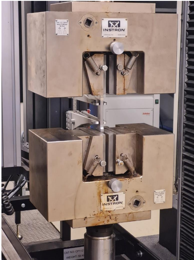
Figure 7 The clamps of the tension test device.
