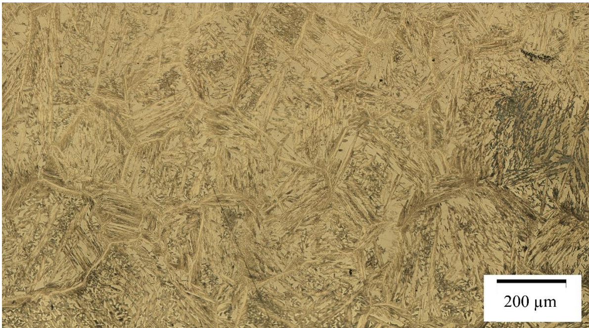
Figure 13 Closer look at the microstructure in the root pass.
