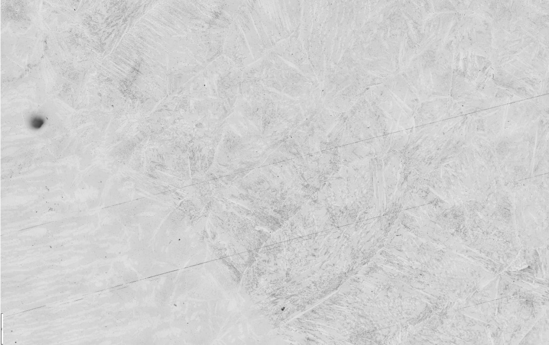
Figure 44 Overview of Side-view sample showing transition from weld to base material.
