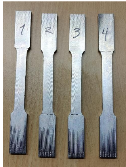
Figure 31: Evidence of gliding in tension test machine
