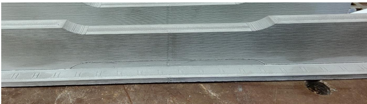
Figure 26: Impurities in the printed specimen
