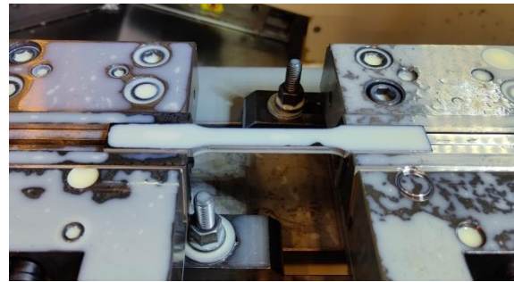
Figure 32: Specimen during machining in CNC
