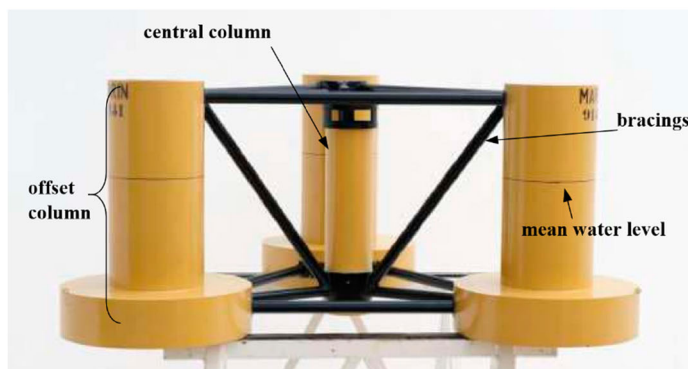
FIGURE 2 Left: DeepCwind semi-submersible floating offshore wind turbine (FOWT) platform 1/50 scale model. 30,32 Right: An example of operating FOWT.
