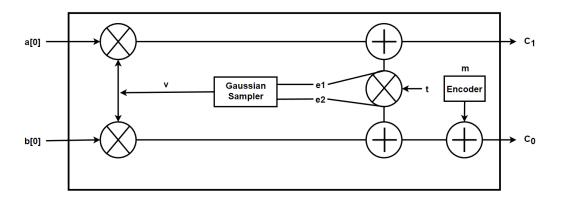
**Figure 2.** Utilizing aggregated public key b[0], shared polynomial a[0] and noise polynomials to encrypt plaintext m into ciphertext tuple ( $c_0$ ,  $c_1$ ). Homomorphic addition and multiplication are represented by "+" and "x" respectively.
