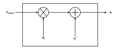
**Figure 3.** How the aggregated  $c_{sum_1}$  is used to compute a partial decryption share  $d_i$  using a client's private key and some added noise. Performed by all clients.
