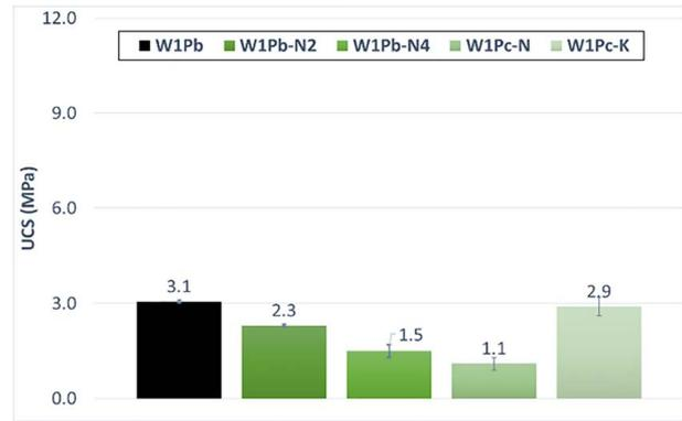
Fig. 5 The effect of NaOH and KOH pellets on 1-day UCS
