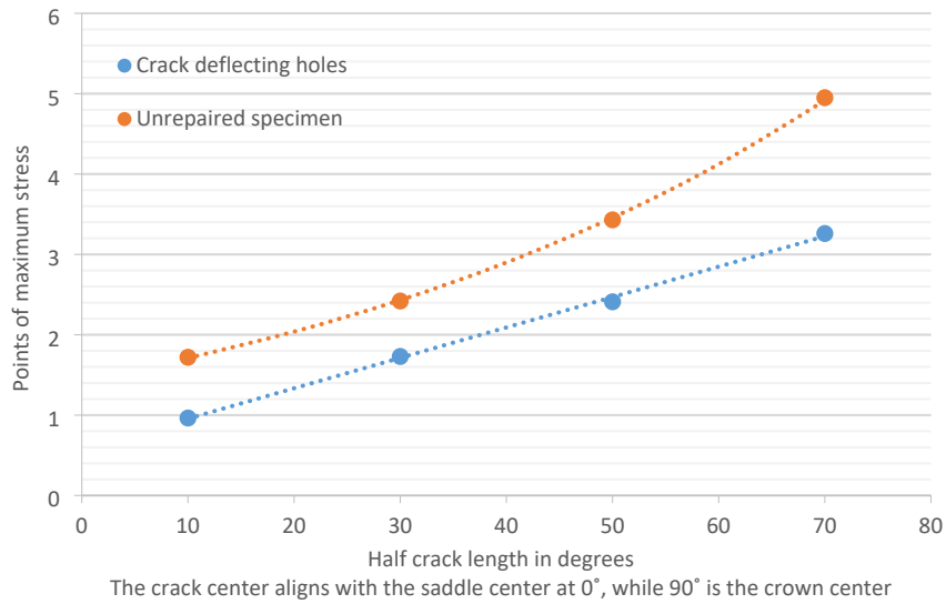
Figure 7-7: Maximum stresses for specimens repaired with crack deflecting holes and unrepaired specimen.
