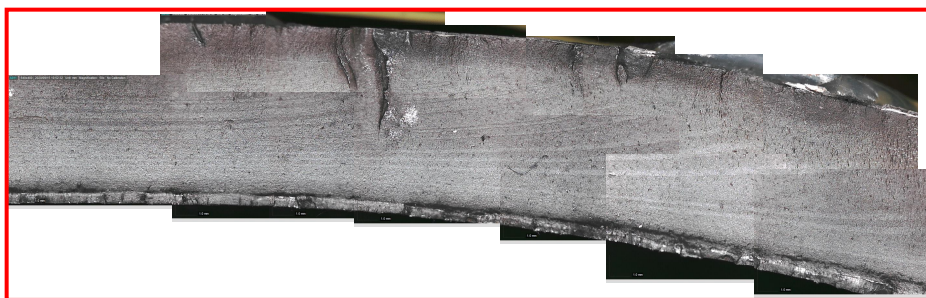
Figure 4-36: Brace/chord crack surface counterpart with rib marks, quadrant 1, Specimen DT1
