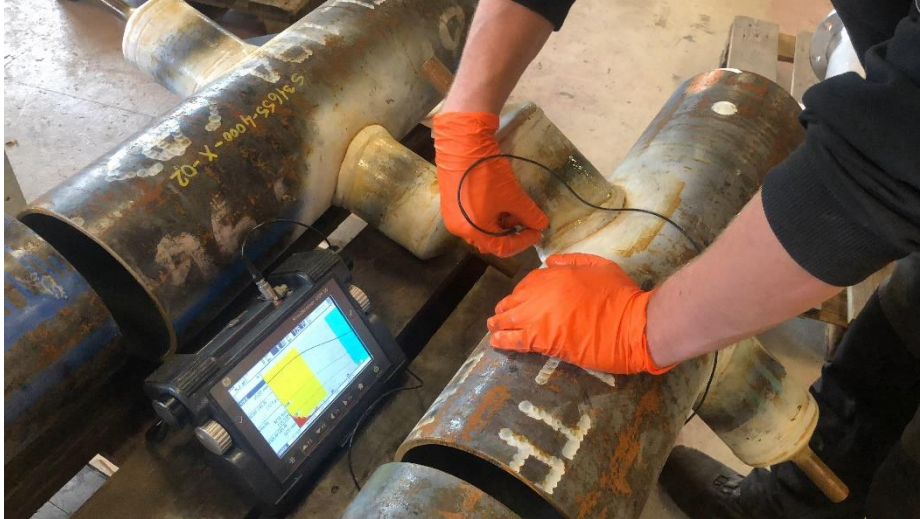
Figure 3-2: ultrasonic non-destructive testing examination.
