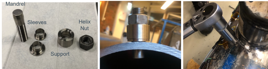
Figure 6-3: Cold expansion process.
