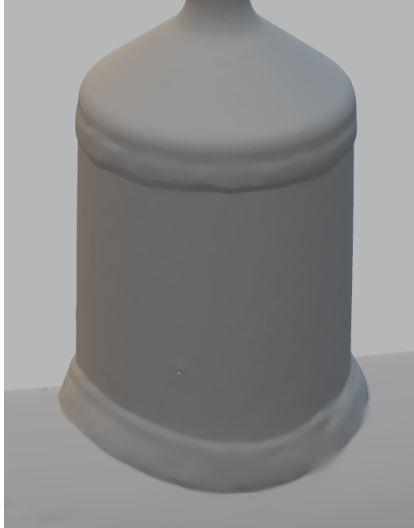
Figure 5-7: A 3D scanned of specimen to illustrate the weld between the brace and chord, brace and cone.
