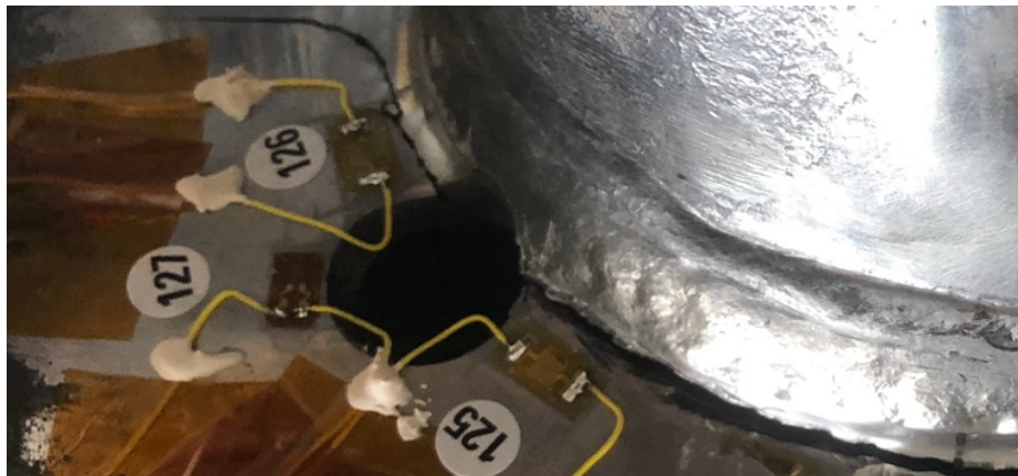
Figure 6-20: Final crack state at the crack-tip hole on quadrant Q3, at the end of the test.
