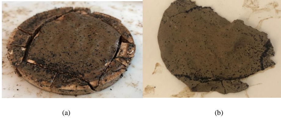
Figure 3-69: Disc from tests of Fluid 2+G+B (a) and reverse side of filter-cake with Granular cellulose seams (b) [IX]
