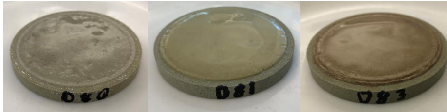
Figure 3-20: From left: Residue from Fluid 1 (Disc 2) after total loss, and filter-cakes from Fluid 2 (Disc 4) and Fluid 4 (Disc 8) [III]
