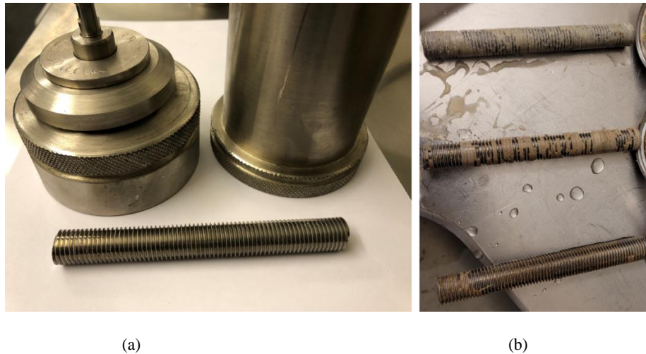
Figure 3-7: 13.5 cm long M16 threaded rod and hot rolling cell (a) and examples of different level of accretion (b)
