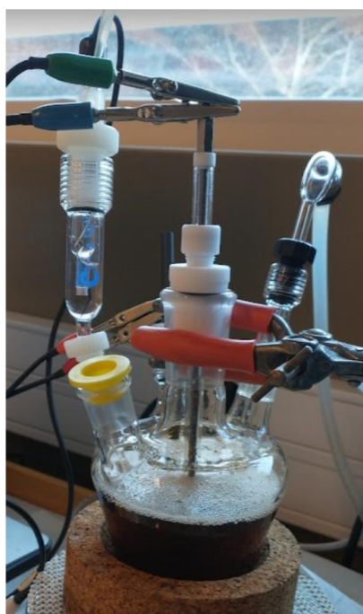
Figure 5. Assembled electrochemical bubble test cell for \text{CO}_2 corrosion inhibitor testing.
