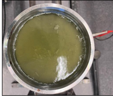
c) gas breakthrough during the hydraulic bond strength test
