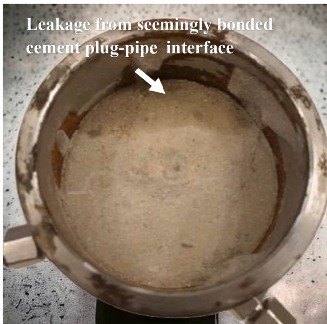
Fig. 1. Leakage at the cement plug-pipe interface (Ogienagbon et al., 2021).
