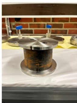
(A) 5-inch casing for Curing of the Slurry
