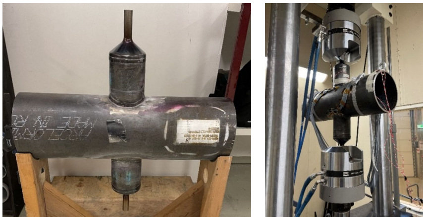
Figure 3. Specimen as-fabricated and installed in fatigue rig, respectively
