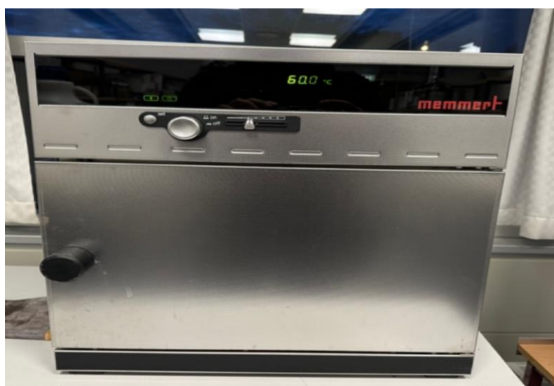
Figure 3.8 The Oven Used for Curing of Plugs
