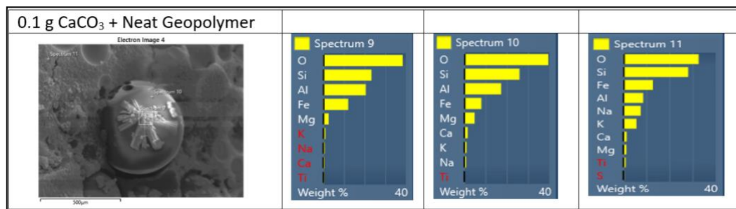
Figure 4.16 EDS Analysis of 0.1 g CaCO 3 Blended Geopolymer
