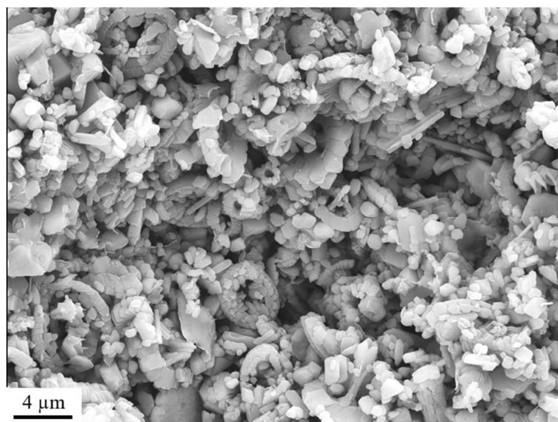
Figure 2. SEM micrograph of Liège chalk showing skeletal debris of coccolithophores and other micro-fossils along with minor occurrences of clay minerals.
