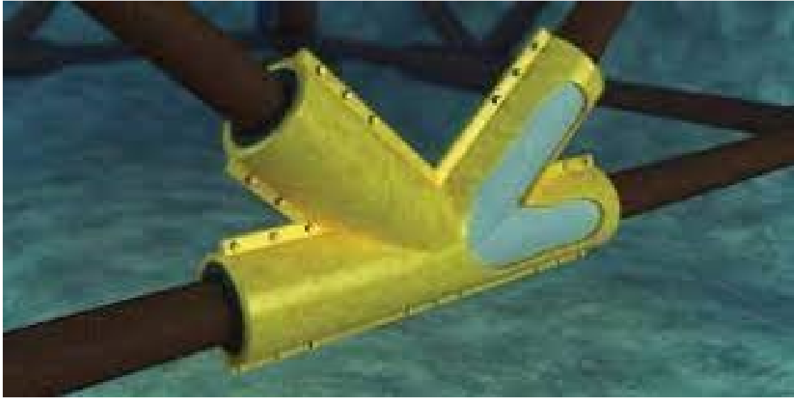
Figure 3-8: Stressed grout-filled clamp (Trident, 2023)
