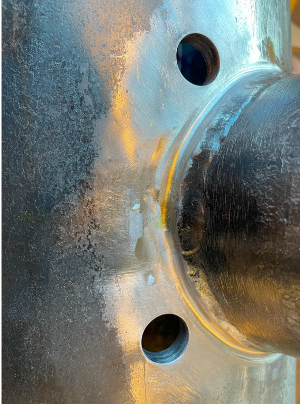
Figure 5-10: Crack deflecting holes
