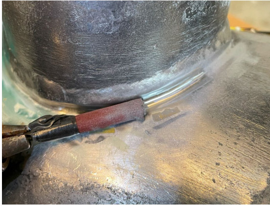
Figure 5-11: Sanding weld toe
