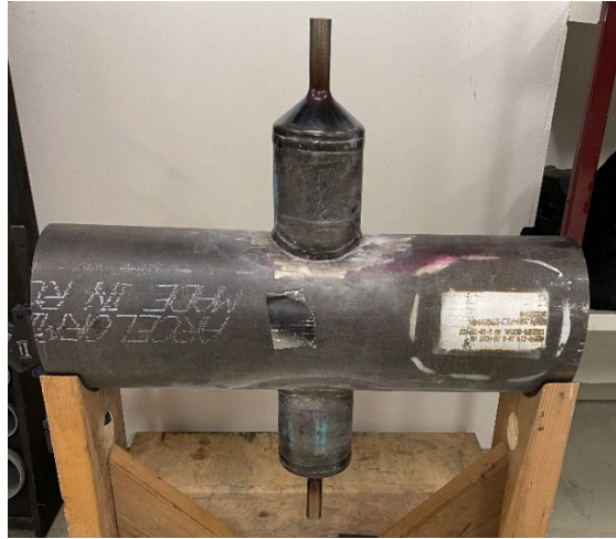
Figure 4-2: DT-joint as built
