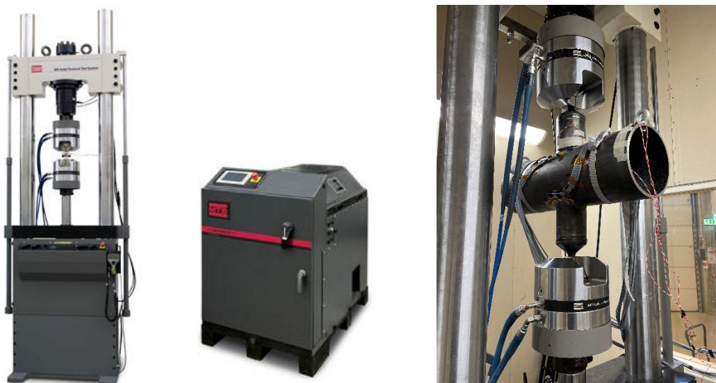
Figure 4-3: Test machine, HPU (MTS, n.d.) and specimen installed in the test system, respectively
