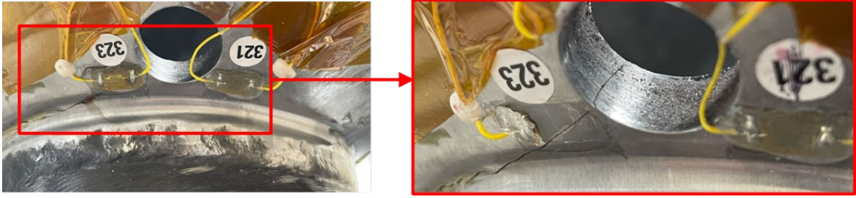
Figure 5-15: Crack propagation into -50° hole
