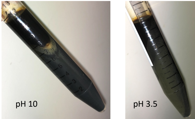
Figure 19 Effect of alkaline (left) and acidic (right) chemical environment on Mongstad sludge
