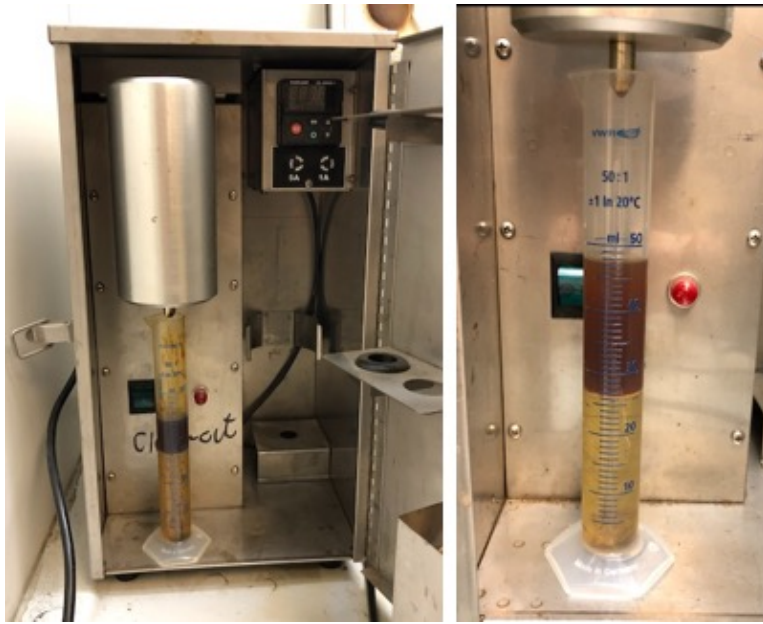
Figure 15 OFITE 50 mL Retort apparatus (left) and the captured liquid fraction after retort analysis (right)
