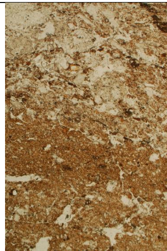
Fig. 2: Photomicrograph of 2022-47-14; silt loam and overlying silty sand layer. Plane polarised light (PPL), frame height is ~4.62mm.
